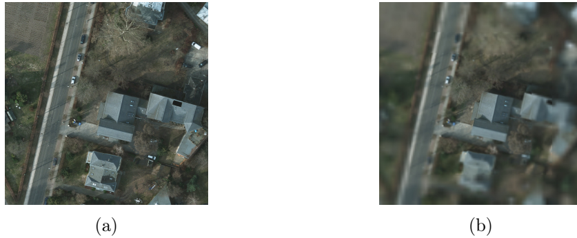
Figure 5.2: To classify the central gray pixel of this patch (and not to confuse it, e.g., with an asphalt road), we need to take into account a spatial context (a). However, we do not need a high resolution everywhere in the patch. It can be lower as we go away from the central pixel and still identify the class (b).
