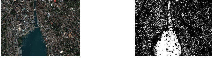
Figure 5.10: A CNN trained on a different dataset misclassifies most of Lake Zurich as a building.
