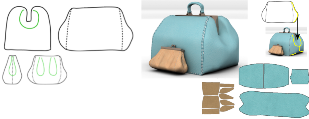
Figure 2.9: The blue purse exhibits non planar silhouette as depicted by the yellow curve.
