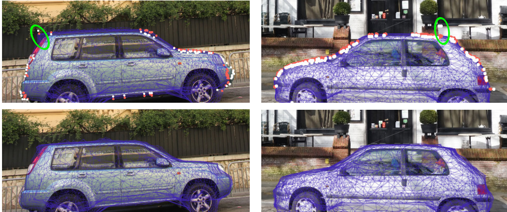
Figure 4.10: Mesh morphing. Because the selected 3D mesh may not correspond exactly to the model in the images, a deformation step is necessary. We use silhouette matching to define constraints on vertices: red points indicate original positions and white points target positions. A multi-view filtering step (see text for details) is necessary to remove remaining outliers (indicated in green). After morphing, the mesh better fits the images and can be used for rendering.
