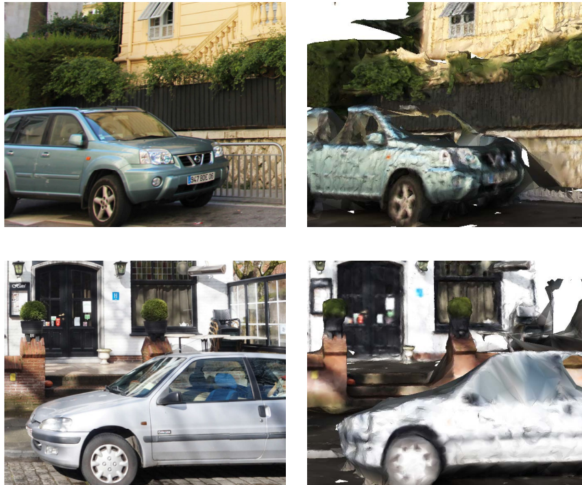
Figure 4.1: MVS reconstruction of specular objects of an urban scene. Left: input view. Right: reconstructed scene.
