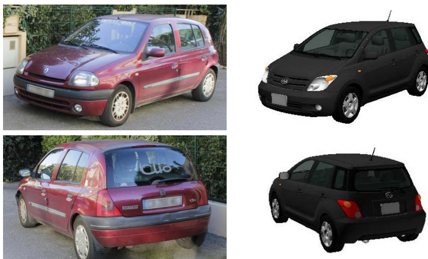
Figure 4.5: Model and orientation matching. The detection algorithm provides 2D bounding boxes for the object. After cropping, the images are used to query the database. Right: the matched rendering which provides both a 3D model and a rough orientation.
