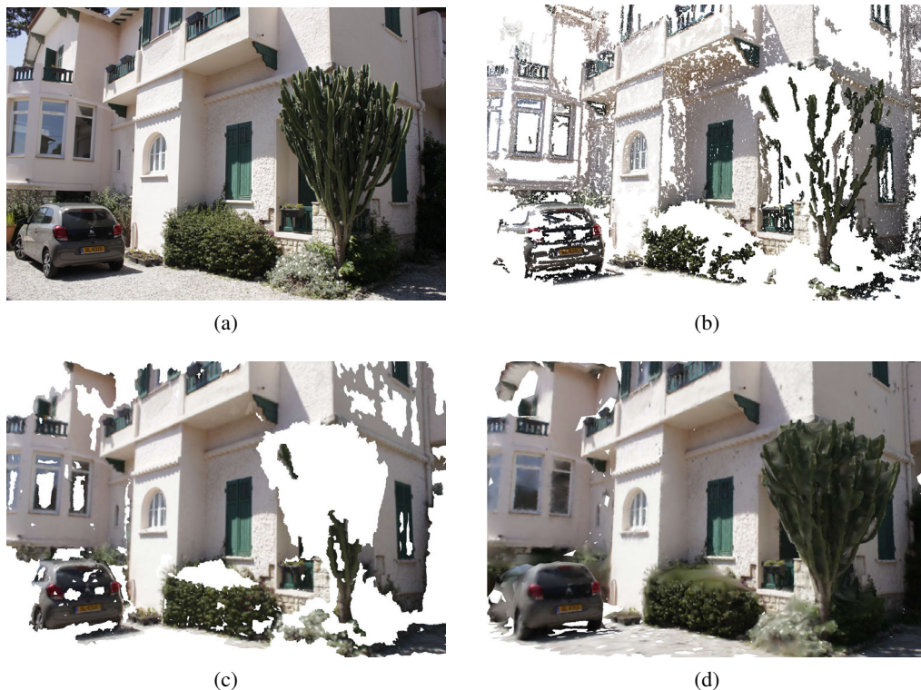
Figure 2.6: Different reconstructions for a 10 view dataset. (a) One out of 10 input images. (b) Point cloud of PMVS reconstruction Furukawa & Ponce (2007) . (c) Mesh of MVE reconstruction Goesele et al. (2007) . (d) Mesh of CPMVS reconstruction Jancosek & Pajdla (2011) .
