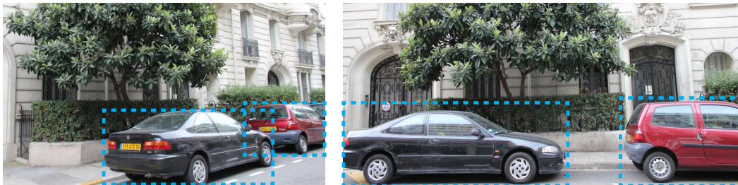
Figure 4.3: Object detection. Using the region aware detection algorithm (Gidaris & Komodakis, 2015) we obtain tight 2D bounding boxes of the objects of interest in the scene.
