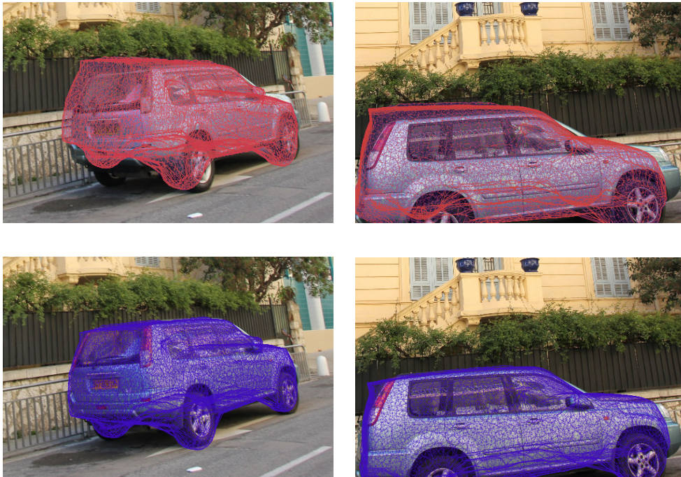
Figure 4.8: Positioning the mesh. Upper row: Initial alignment for two views; Bottom row: fine-grain alignment.
