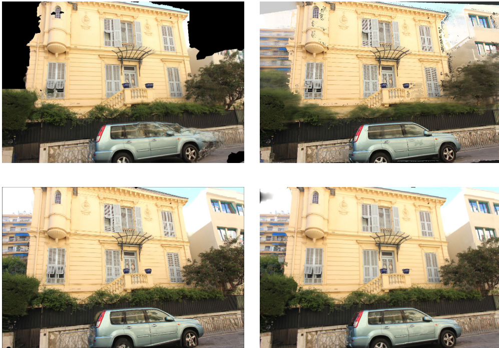
Figure 2.11: Novel view rendered with 4 previous methods. Top-left: Floating textures of Eisemann et al. (2008) . Optical flow fails in specular regions like the front of the car. Top-right: Ambient point clouds of Goesele et al. (2010) . Regions with no depth (upper corners of the image) are sampled with multiple depth pixels. Bottom-left: Silhouette-aware warping of Chaurasia et al. (2011) . Regions around the car present distortion. Bottom-right: Shape-preserving warping of Chaurasia et al. (2013) . A complete and plausible image is generated, however, the car and the facade present artifacts.
