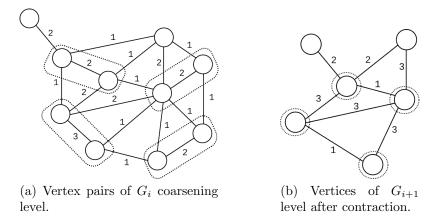
Figure 2.4: Contraction of egdes in HEM. Note how the edge weights are updated after the contraction of vertices. Vertex weights are not illustrated
