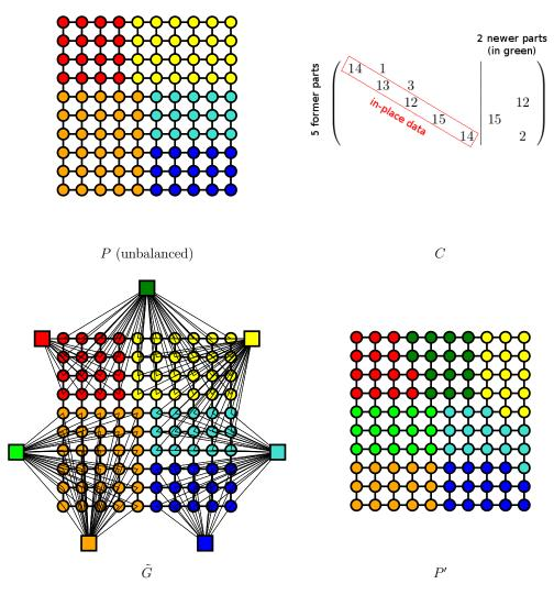
Figure 4.6: Sample of a  $5 \times 7$  repartitioning of a 2D grid of dimensions  $10 \times 10$ . The migration matrix C explains how vertices will migrate from the 5 former parts to the 7 newer. It is chosen to minimize both totZ and totV. On the enriched graph  $\tilde{G}$ , the square vertices represents the l fixed vertices, connected to former parts according to C. The final partition obtained is well balanced and respects the communication scheme imposed by C.
