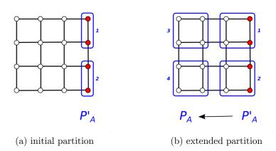
Figure 4.7: Given the  $k'_A$ -way partition  $P'_A$  of  $G'_A$  in Figure 4.7a, the extension operator computes a  $k_A$ -way partition  $P_A$  of  $G_A$  in Figure 4.7b, with  $k'_A = 2$  and  $k_A = 4$ .
