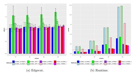
Figure 3.9: KGGGP evaluation on the Walshaw collection relatively to SCOTCH, without multilevel framework. Comparison of the three gain formulas (*classic*, *diff* and *hybrid*) for a parameter  $\alpha$  equal to 1 or 10, and comparison of the *global* and *local* version of KGGGP.
