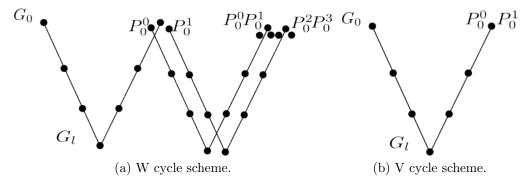
Figure 2.5: Illustration of the multilevel framework.
