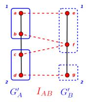
Figure 4.8: Illustration of the projection operator from graph  $G'_A$  to  $G'_B$ . Given the  $k'_A$ -way partition  $P'_A$  (in blue), one aims to find a  $k'_A$ -way partition of  $G'_B$  (in dashed blue), with  $k'_A = 2$ .
