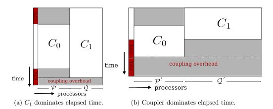
Figure 2.13: Two examples of the fully concurrent execution of components for the sequential CCS (where  $\mathcal{P} \neq \mathcal{P}', \mathcal{Q} \neq \mathcal{Q}'$ ). In 2.13a the coupling overhead is partially hidden, as opposed to 2.13b.
