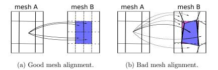
Figure 4.18: Examples of different mesh alignment in the coupling interface.
