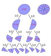
Figure 3.1: Illustration of the RB method: bisection tree and its implicit part numbering (in red) for a 8-way partition.
