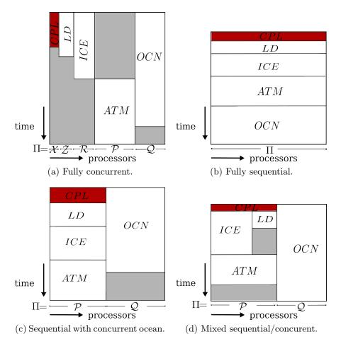
Figure 2.14: Four different processor layouts for the coupled simulation of earth's climate. Each figure is an example of one iteration for the coupled simulation.
