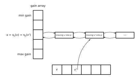
Figure 2.3: Gain bucket structure introduced in FM algorithm.  $s_p(v)$  defines the gain function of moving vertex v into part p
