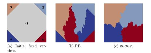
Figure 3.2: Given initial fixed vertices, comparison of two different partitioning methods (RB and KGGGP). Results of a 4-way partition of a  $1000 \times 1000$  grid graph: the RB method fails to extend an initial partition while the KGGGP method succeeds.
