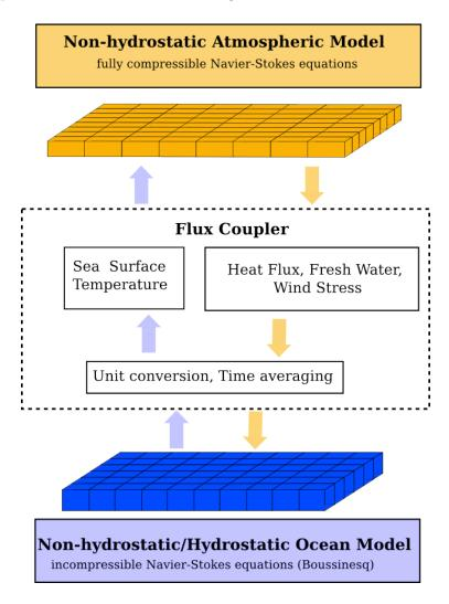
Figure 2.8: Coupling between atmospheric and ocean model.
