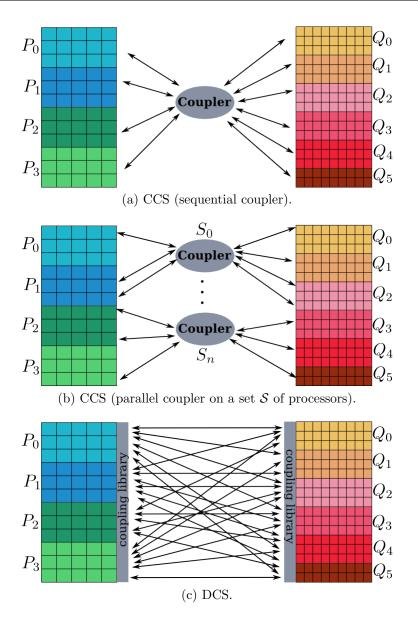
Figure 2.7: Different communication schemes for coupling component models with different mesh resolutions and different partitions on sets  $\mathcal{P}, \mathcal{Q}$  respectively.
