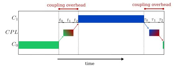
Figure 2.12: Coupling overhead within the CCS when components run sequentially in time. Example of one iteration.
