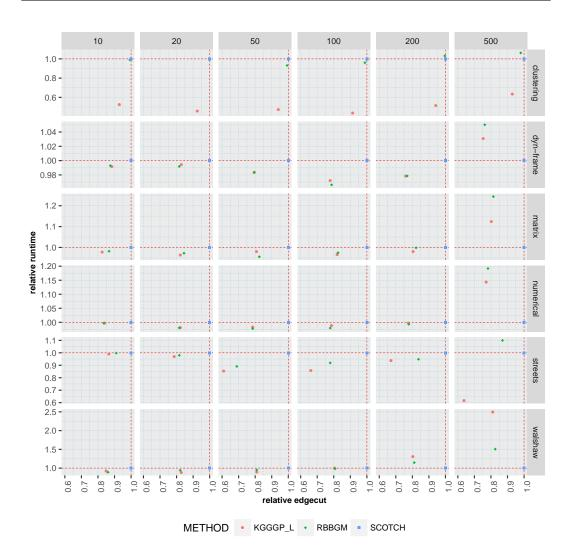
Figure 3.14: Average results on the edgecut quality and time execution for each group in the *DIMACS'10* collection (*bubble* scheme).
