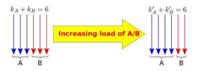
Figure 5.1: Dynamic processor allocation for two components A and B whose relative load A/B increases.
