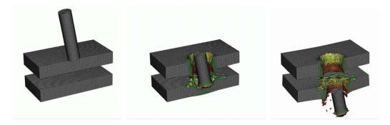
Figure 4.3: Example of contact-impact simulation (extracted from [41]).
