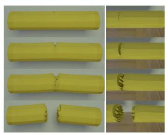
(c) A cut that results in a propagating crack
