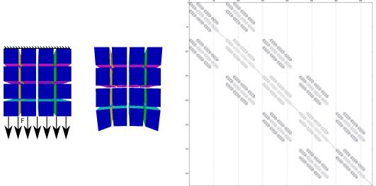
**Figure 3.5:** Sparsity of a stiffness matrix in an example of a hexahedral beam: *left* example in initial configuration with forces on bottom (*black arrows*) and fixed displacement conditions on top; *middle* deformed configuration; *right* entries in the stiffness matrix
