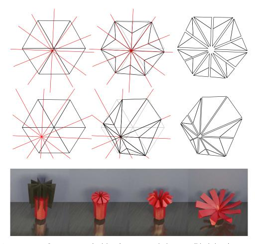
Figure 5.17: Crossing cuts (red lines) over several elements (black lines) using our re-meshing approach combined with the snapping of nodes; intersection of cuts close (top row) and far (middle row) to mesh node; results in three dimensional case (bottom row)
