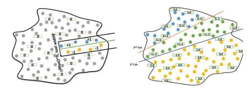
Figure 4.4: Labeling of the nodes ((pair of) numbers close to nodes) when virtual cuts occur (figure extracted from [104])
