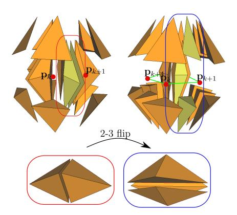
Figure 5.2: A set of tetrahedra before (top left) and after (top right) the 2-3 flips. Flipping the faces incident to e creates a closed polygon  $\{\mathbf{p}_k, \ldots, \mathbf{p}_{k+n(v(e))}\}$  (green); (bottom) 2-3 flip of two tetrahedra.
