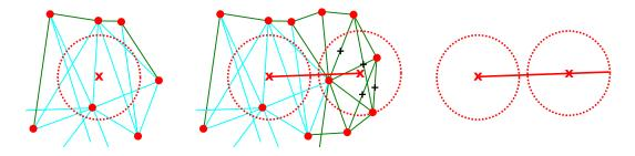
Figure 7.7: Left: removed connectivity information (turquoise) in circle around new cut point (red cross); Middle: insertion of a second cut point yields a cut line (polygon) (red line); Right: cut polygon is extended until the end of its radius  $r_{\mathbf{p}_c}$
