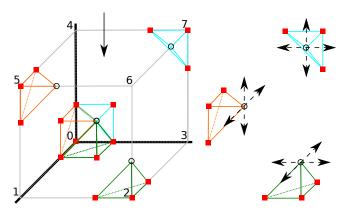
Figure 3.10: Example of locking behaviour in 3D: cube (grey lines) is fixed for all faces containing the node 0 and undergoes load (black arrow) equally distributed on top face (face with nodes 4,5,6,7); plot of three different tetrahedra types with fixed nodes (red squares) and possible movements (black arrows with dashed lines)
