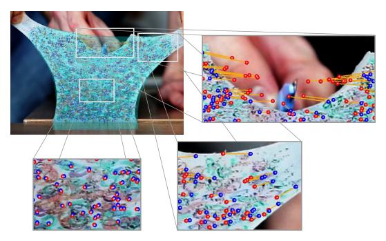
Figure 7.5: Effects of topological changes in image on virtual object (turquoise) with target (blue dots) and current features (red dots) connected by springs (orange lines): Top left: complete object with overlayed virtual object; Top right: cut region; Bottom left: region without strong deformation; Bottom right: region with strong deformation
