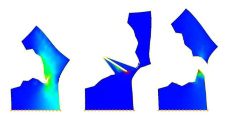
Figure 6.16: Fracture of a thin sheet without snapping (*left*) and with snapping (*middle*, *right*). Without (*middle*) and with (*right*) transforming the fracture direction in the undeformed configuration
