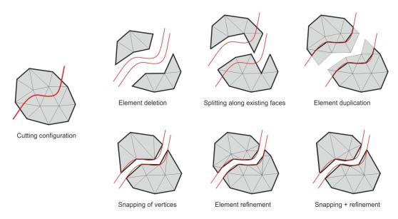
Figure 4.1: Two dimensional illustration of the different methods for the incorporation of a cut *(red curves)* into a mesh, with the boundary depicted as a *black bold line* (figure extracted from [128])
