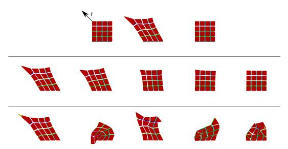
Figure 3.4: First line: Considered example left rest position with applied forces, middle deformed position when force is set to zero, right expected final position; Relaxation process shows different behaviour when using an implicit (second line) and explicit euler method (third line) that is unstable and explodes at the end
