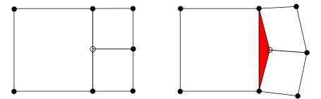
Figure 3.13: Hanging node: *Left*: initial configuration, the *hollow black dot* is only present in the smaller elements; *Right*: when staying untreated, the node in the middle *(hollow black dot)* can move freely introducing a gap between elements *(red triangle)*
