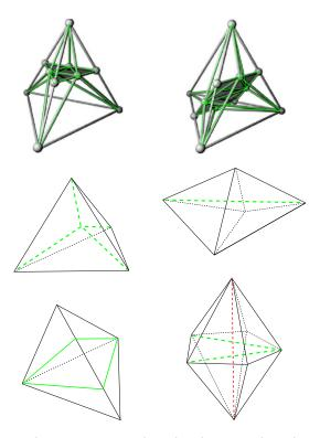
**Figure 6.7:** Topological operations used in the theoretical analysis with newly inserted edges in *green* and deleted edges in *red*: *Top*: Bielser three cut edges and four cut edges (figures taken from [13, 14]); *Middle*: Split 1 to 4 and flip 2 to 3; *Bottom*: 2 node insertion (applied in [50]) and general flip
