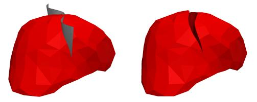
**Figure 4.7:** A liver with 888 linear tetrahedral elements is cut by a sinusoidal blade (figure extracted from [77]): undeformed with the cutting surface (*left*), and deformation after the cut (*right*)
