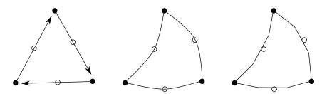
**Figure 6.1:** Quadratic triangle representations: *Left:* topological, with vertex ids saved as edge attributes; *Middle:* continuous representation; *Right:* visualization using tesselation
