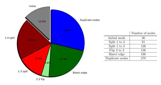
**Table 6.5:** Cut of quadratic liver (see figure A.28), impact of the different topological operations on the number of nodes: *Left:* pie chart; *Right:* table with the added nodes after the subsequent operations
