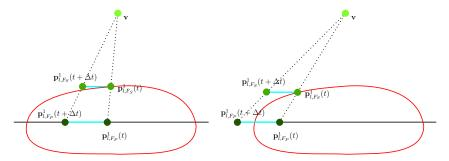
Figure 7.3: Calculation of the virtual features using the intercept theorem, with the projection plane (black line), the object (red curve), the camera position  $\mathbf{v}$  and the rays defining the virtual features (dashed black lines)
