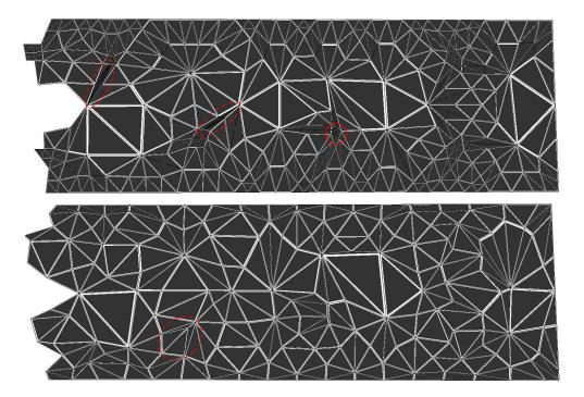
Figure 5.12: The separation surface: (top) with Bielsers approach; (bottom) with our re-meshing method; small triangles and thus potentially small tetrahedra are surrounded by a  $(red\ circle)$ , sliver triangles and thus potetially illshaped tetrahedra are surrounded by  $(red\ dashed\ ellipses)$
