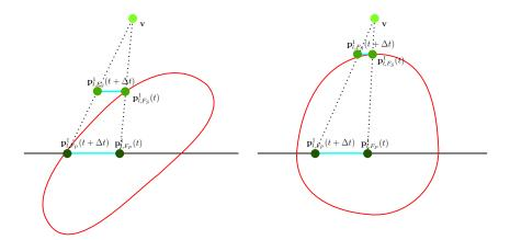
Figure 7.4: Virtual features on thin object non-perpendicular to the camera (left) and a thick object (right), with the projection plane ( $black\ line$ ), the object ( $red\ curve$ ), the camera position v and the rays defining the virtual features ( $dashed\ black\ lines$ )
