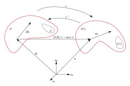
Figure 2.1: Motion of a continuum body with deformation of the object
