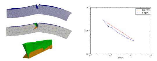
Figure 4.6: Convergence analysis displaying the root mean square error (right) of the eXtended FEM compared to a perfectly aligned conventional FEM solution on an example of a cut in a beam (figure extracted from [77]): reference solution (left top), solution with 1810 elements and 595 nodes (left middle), zoom on partially (orange) and completely (green) cut elements (left bottom)
