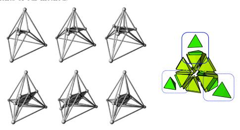
**Figure 5.9:** Reference re-meshing algorithms: *Left:* 1:17 subdivision (figure extracted from [13]); *Right:* one step of the re-meshing algorithm proposed by [50] (figure extracted from [50])
