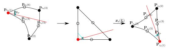
**Figure 6.14:** Calculation of the fracture direction in the material configuration: *Left:* calculation of the intersection between a curve inside an element with the fracture direction in spatial configuration to obtain the barycentric coordinates of the point *(middle)*; *Right:* fracture direction in material configuration
