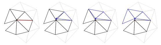
Figure 4.8: Separation process on the topological level for linear elements: intended separation direction (red dotted line/curve) and node to be duplicated (black dot), duplication of node (blue dot): before topological change (left), at node duplication and the update of direct neighbors of the edge (middle left) and the update of elements sharing the node (middle right and right)
