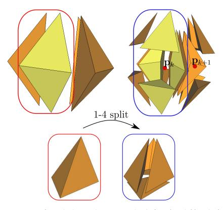
Figure 5.1: A set of tetrahedra incident to an edge before (top left) and after (top right) the 1-4 split; (bottom) 1-4 split of a tetrahedron.
