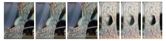
Figure 7.12: Detection and simulation of cuts in silicone bands demonstrating the ability of our approach to distinguish between large strains (186% and 166%) and cuts, augmented with an uncut/cut model (edges are plot as white lines)
