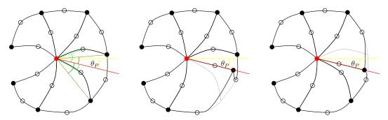
**Figure 6.13:** Snapping of quadratic triangles to a fracture direction (red line) that starts from a node with the maximal principal stress  $\sigma_{P,+}$  (red dot): Left: comparison of angles between edges and fracture direction (different approaches in green); Snapping of lower (middle) (and respectively upper (right)) edge, based on criteria presented in light green (and respectively dark green) on the left
