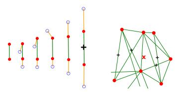
Figure 7.6: Left: Neighboring features: From left to right initial position, increasing measure, an identified outlier (black cross); Right: Initialization of a cut point as the weighted barycenter of the outliers (black crosses); Target (blue dots) and current features (red dots) are connected by springs (orange lines), the neighborhood information between two features displayed in green
