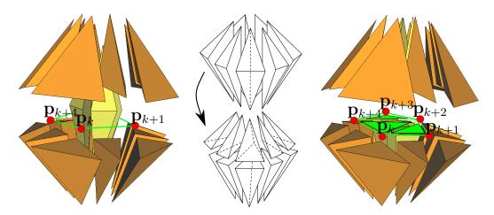
Figure 5.3: (*left*) tetrahedra surrounding the cut edge (*yellow*); (*middle*) general flip; (*right*) triangulation of the separation surface (*green triangles*), showing the tetrahedra below the cut
