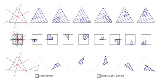
Figure 5.16: Comparison of different cutting algorithms when crossing cuts (red lines) occur; First row: virtual node algorithm; Second row: Composite finite element method, links in green; Thrid row: our re-meshing approach combined with the snapping of the nodes ToDraw: improve the visualization of visual and computational elements (later)
