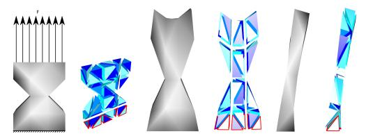
Figure 3.11: Example for an unrealistic behaviour due to volume locking: locked elements are surrounded by *red lines*; *from left to right*: initial configuration with applied forces on top and fixed boundary condition on bottom, mesh in initial configuration, final configuration front view, mesh in final configuration front view, final configuration side view, mesh in final configuration side view
