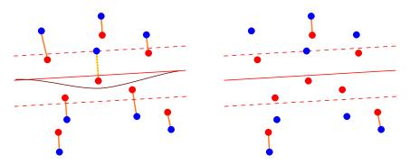
Figure 7.8: Left: Example of a detected cut (red line) that would be closed due to a spring intersecting with the cut (yellow dashed line), the actual cut is plot in dark red, target features (blue dots) pull the current features (red dots) with the springs (orange lines) away from the cut; Right: springs are removed in margin (dashed red lines) around the detected cut
