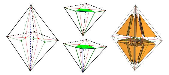
Figure 5.6: Re-meshing around a boundary edge (dotted blue line). (left) 1-4 splits are applied to all tetrahedra (new edges are plot as red lines), next 1-3 splits are applied on the boundary tetrahedra only (new edges are plot as green lines); then, the boundary edge is replaced by a general flip (middle top) or split to maintain a desired feature (middle bottom); (right) the final re-meshing on the boundary of the object after a split of the edge.
