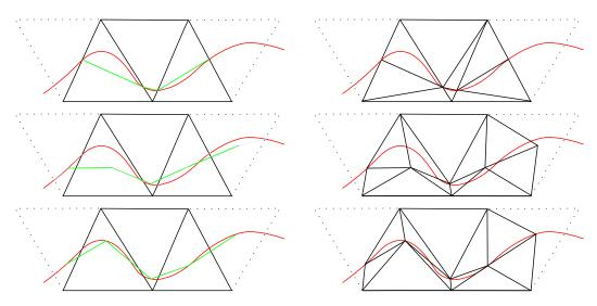
**Figure 5.13:** Approximation of a cut (red curve) inside a mesh (black lines) using different sampling and re-meshing ideas, before the re-meshing (left) and after the re-meshing (right): Top row: sampling and re-meshing on the edges; Middle row: sample nodes chosen on the edges but placed inside the element Bottom row: sampling and re-meshing inside the element
