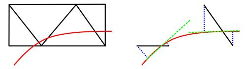
Figure 5.7: Left: Cut (red curve) of a triangular mesh (black lines); Right: Intersected edges (black lines), with the slope of the cut curve at the intersection (dotted green lines), and the distances to the edge vertices (dotted blue lines)
