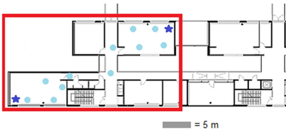
FIGURE 3.10: Experimental area map at the Institute for Technical Informatics of the Graz University of Technology. The source and the sink nodes are represented by dark blue stars, whereas the intermediate nodes are represented as blue spots. Credits: Carlo Alberto Boano
