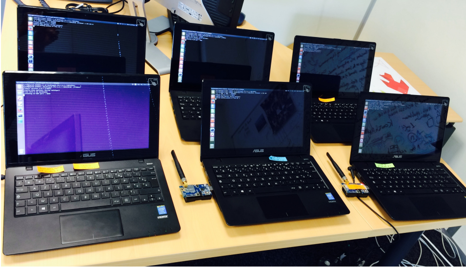
FIGURE 3.6: Experimental setup: 3 pairs of laptops occupy 3 orthogonal channels of Wi-Fi (1, 6, 11)
