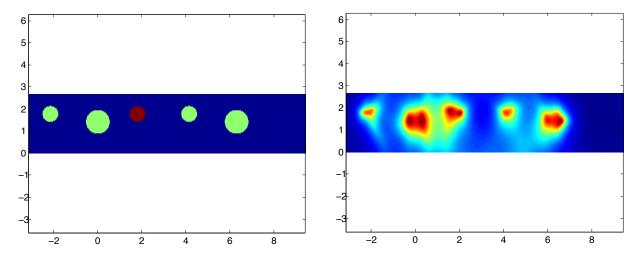
Figure 4.14: Left: The exact geometry for Example 3. Right: the reconstruction of this domain using  $z \mapsto \mathcal{I}^{\text{GLSM}}(z)$ .
