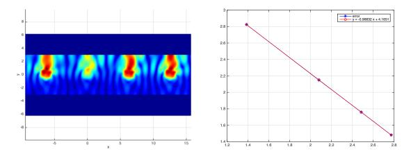
Figure 3.8: Left: Illustration of the scattered wave in  $\Omega_{M_0}$ . Right: The relative error in  $\Omega_{M_0}$  with respect to M. The geometry of the experiment is shown in Figure 3.5
