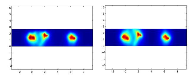
Figure 4.11: Reconstructions of the full domain  $D_p \cup \omega$  using GLSM. The exact geometry is shown in Figure 4.10. From left to right:  $z \mapsto \mathcal{I}_+^{\text{GLSM}}(z)$  and  $z \mapsto \mathcal{I}_-^{\text{GLSM}}(z)$
