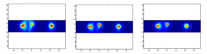
Figure 4.3: Reconstruction of the domain  $D = D_p \cup \omega$  using, from left to right,  $\mathcal{I}_+^{\mathrm{LSM}}(z)$ ,  $\mathcal{I}_-^{\mathrm{LSM}}(z)$  and  $\mathcal{I}_-^{\mathrm{LSM}}(z)$ .
