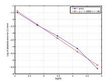
Figure 3.7:  $L^2(\Omega_0^h)$  norm of  $u_M^{R,N} - u_M^{R,N_{\max}}$  where  $N_{\max} = 2^{11}$  and  $N = 2^n, n = 3, \dots, 7$  in the case of locally perturbed periodic media and piecewise constant refractive index.
