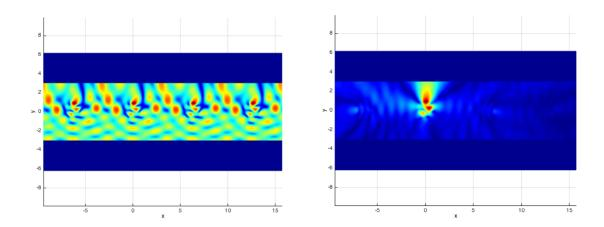
Figure 3.14: Left: The background total field  $u_p$  in  $\Omega_{M_0}$  for real  $n_p$ . Right: The scattered field  $\tilde{u}^s$  in  $\Omega_{M_0}$  for real  $n_p$ . The geometry of the experiment is shown in Figure 3.5
