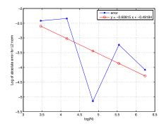
Figure 3.3: Left: The rate of convergence of  $E_N$  with respect to N when evaluating the convolution operator using exact Fourier coefficients. The rate of convergence of  $\tilde{E}_N$  with respect to N when evaluating the convolution operator using FFT.
