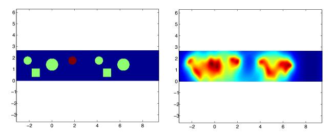
Figure 4.16: Left: The exact geometry for Example 4. Right: the reconstruction of this domain using  $z \mapsto \mathcal{I}^{\text{GLSM}}(z)$ .
