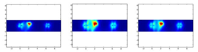
Figure 4.9: Reconstruction the local perturbation  $\omega$ . The exact domain configuration is shown in Figure 4.2. From left to right:  $z \mapsto \mathcal{I}^{+,\delta}(z)$ ,  $z \mapsto \mathcal{I}^{-,\delta}(z)$  and  $z \mapsto \mathcal{I}^{\delta}(z)$
