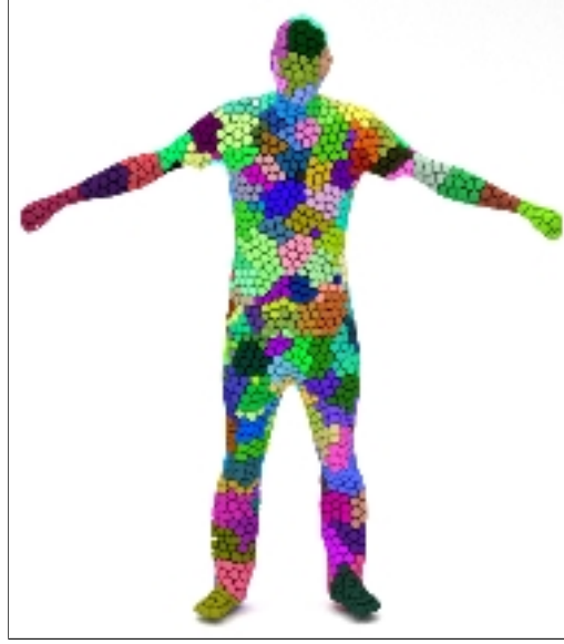
Figure 6.6 – The template model used to recover the runner sequence motion, with its CVT decomposition cells, and the cell clusters in different colors.
