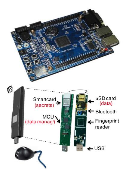
Figure 18: The development board ST3221G-EVAL used in the experiments (above) and the real hardware plateform (below).
