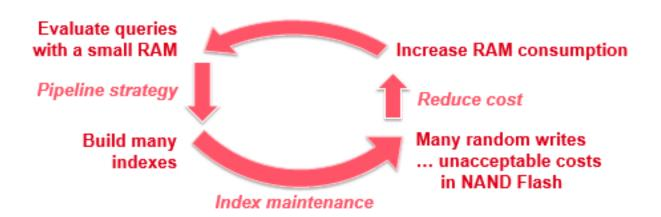
Figure 9: Tiny RAM and large NAND flash storage lead to conflicting constrains
