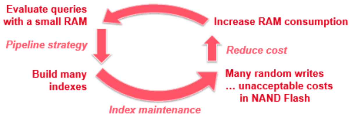
Figure 9: Tiny RAM and large NAND flash storage lead to conflicting constraint
