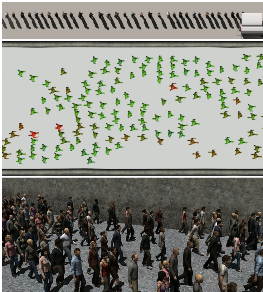
Figure 3.5 Two scenarios. Top: waiting line scenario simulating 1-D following traffic. Center: top view of the periodic corridor simulating 2-D following traffic by using an overtaking rule. The agents in red are walking fast, they will slow down when facing agents blocking their way and try to overtake them. Bottom: perspective view of the periodic corridor.
