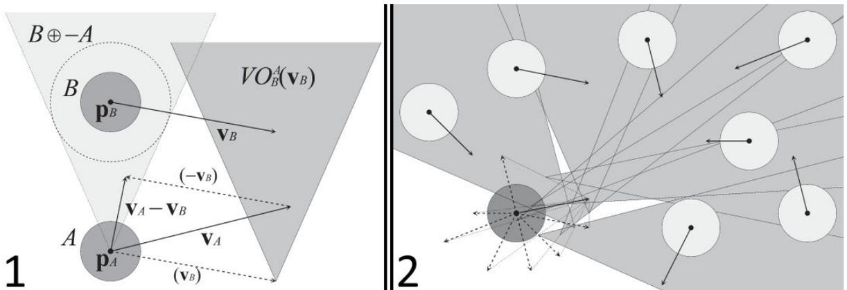
**Figure 2.2** On the left, the computation of the velocity obstacle of agent A that leads to a collision with agent B. On the right, the union of all the velocity obstacles to avoid multiple obstacles.
