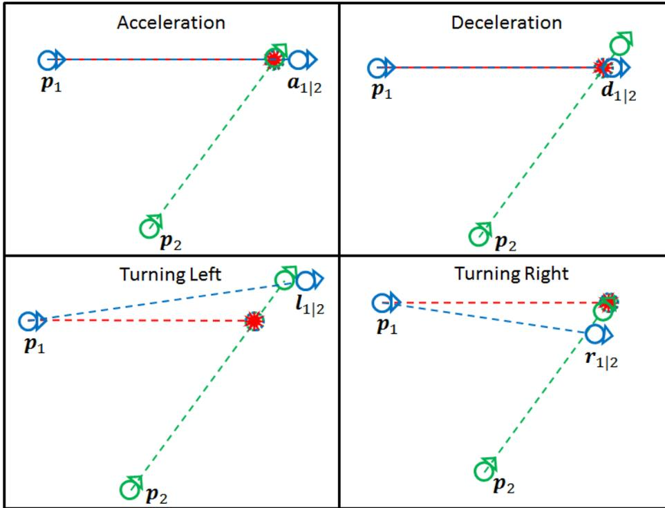
**Figure 4.4** Example of collision solved using the four CIW. The collision trajectories are drawn in red and the four trajectories followed to reach the CIW are shown in blue. The position of each CIW is shown together with the position of the other agent when the CIW is reached.
