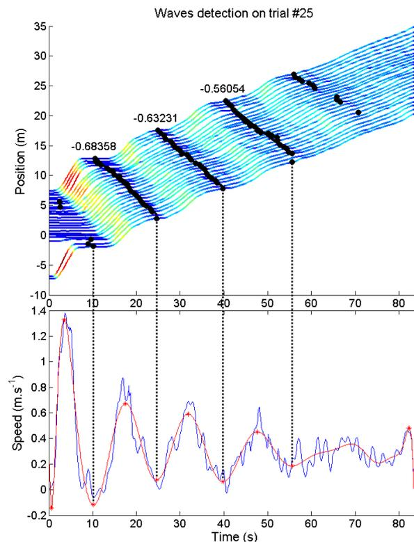
**Figure 3.8** Waves detection on trial #25 of the real trajectories database. The upper plot shows all the trajectories with the detected minima as black stars and the defined waves propagation as black lines. The lower plot shows the speed of the last person in blue, the smooth speed in red and the detected extrema as red stars.
