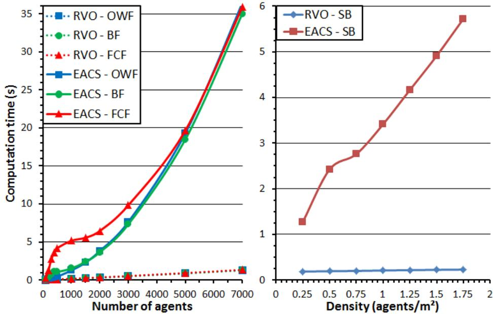
**Figure 4.9** The graphs show the time needed to compute 20 seconds of simulation for the different performance test situations with and without EACS. On the left graph, the results of the three situations: OWF, BF and FCF are presented for different numbers of agents. The right graph presents the results of the SB situation for different densities.
