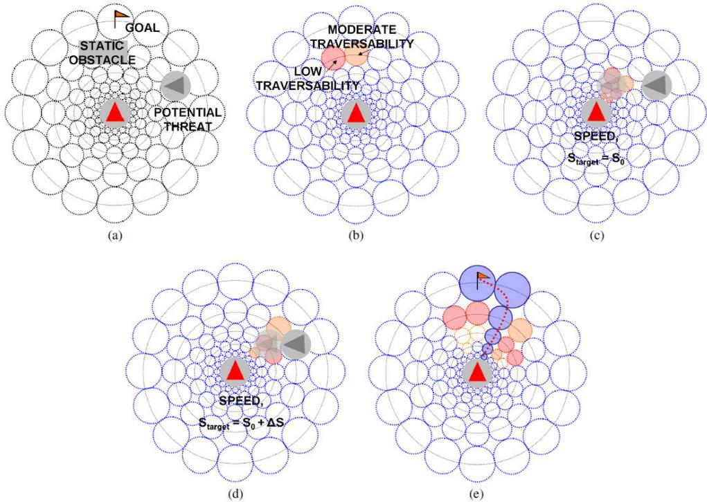
**Figure 2.7** The steering algorithm of the Egocentric Affordance Fields [KSHF09]: (a) The current state of the environment. (b) Static Perception Field indicating low traversability at position of obstacles. (c) Dynamics Perception Field for velocity,  $S_{target} = S_0$ . (d) Dynamics Perception Field for velocity,  $S_{target} = S_0 + \delta V$ . (e) Affordance Field indicating path of high fitness to goal.
