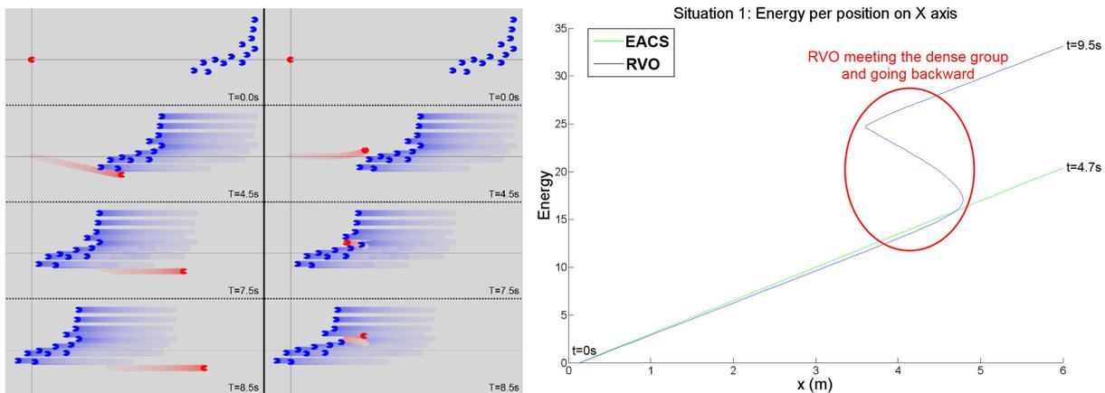
**Figure 4.13** Left: simulated test where short-term cost leads to bad mid-term cost, agents simulated with EACS on the left and without on the right. Right: the graph quantifies the energy consumption of the red agent (For RVO2 and EACS) as they walk towards the goal (In this situation, it is equivalent to the distance traveled on the x axis). The section of the blue curve circle in red corresponds to RVO2 agents going backwards to avoid the dense group (T=7.5s on the top figure).
