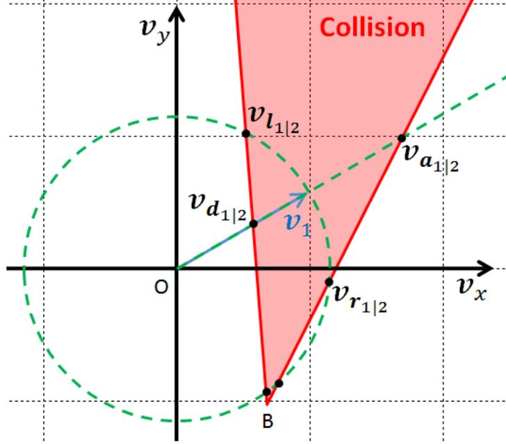
**Figure 4.3** Collision velocity space for one interaction, in red.  $\mathbf{v}_{a_{1|2}}$ ,  $\mathbf{v}_{r_{1|2}}$ ,  $\mathbf{v}_{d_{1|2}}$  and  $\mathbf{v}_{l_{1|2}}$  represent the collision-free velocities that are used to compute the CIW.
