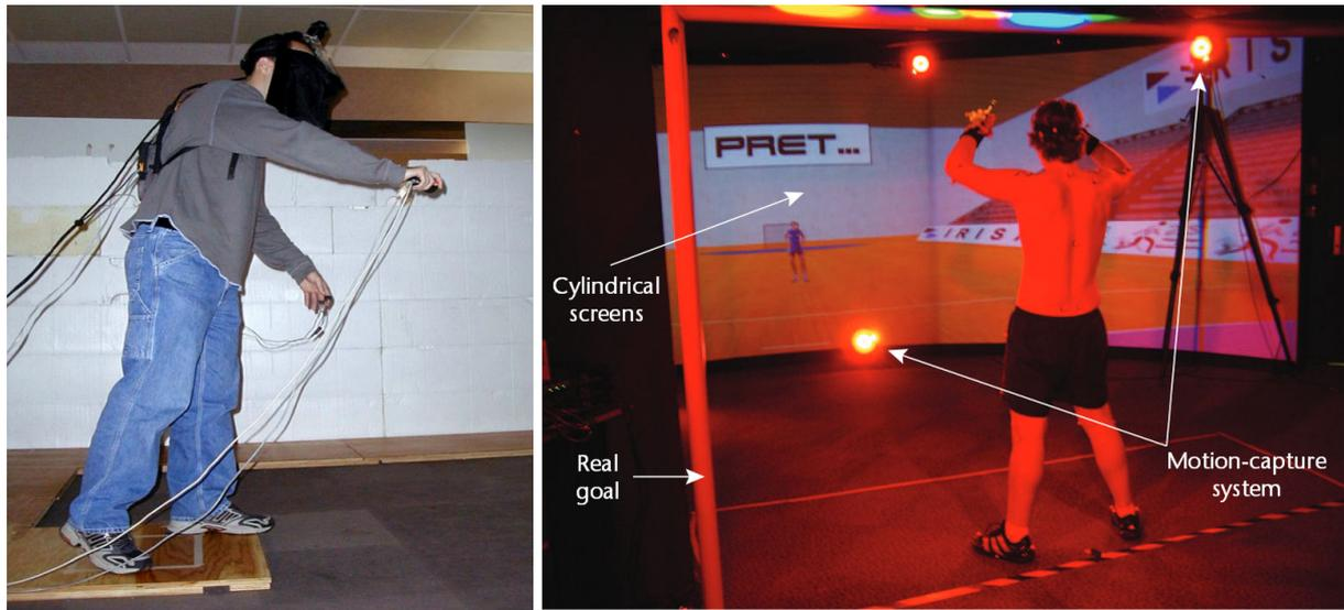
**Figure 2.17** Left: subject wearing HMD and physiological monitoring from the experiment in [MIWB02]. Right: subject in a cave facing a virtual thrower in the handball case study from [BKV<sup>+</sup>10].
