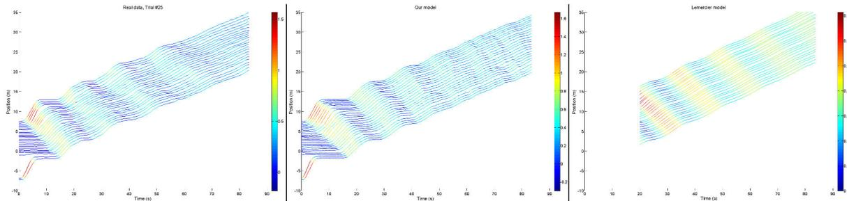
**Figure 3.6** Trajectories from experiment trial #25 (left) and the simulation results from our model (center) and Lemerrier’s one (right). Lemerrier’s model needs some initial motion to work so it has been initialized after  $20 \text{ s}$  of real motion. In our model, we just need to place the walkers at the initial positions extracted from the real data.
