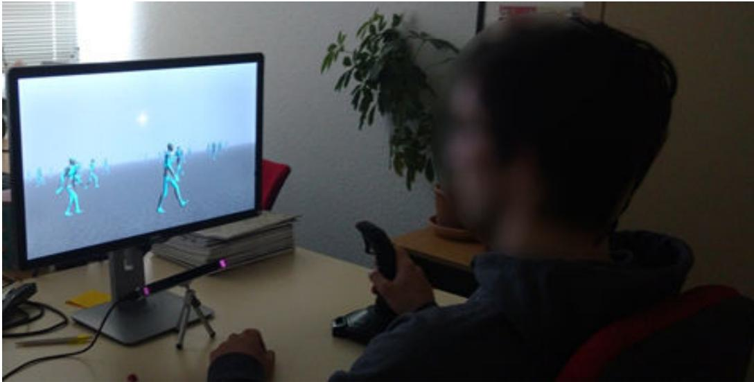
**Figure 6.5** Participant using the joystick to navigate in the virtual environment while his eyes are being tracked by the eye tracking device below the screen (the captor with purple dots on each side).
