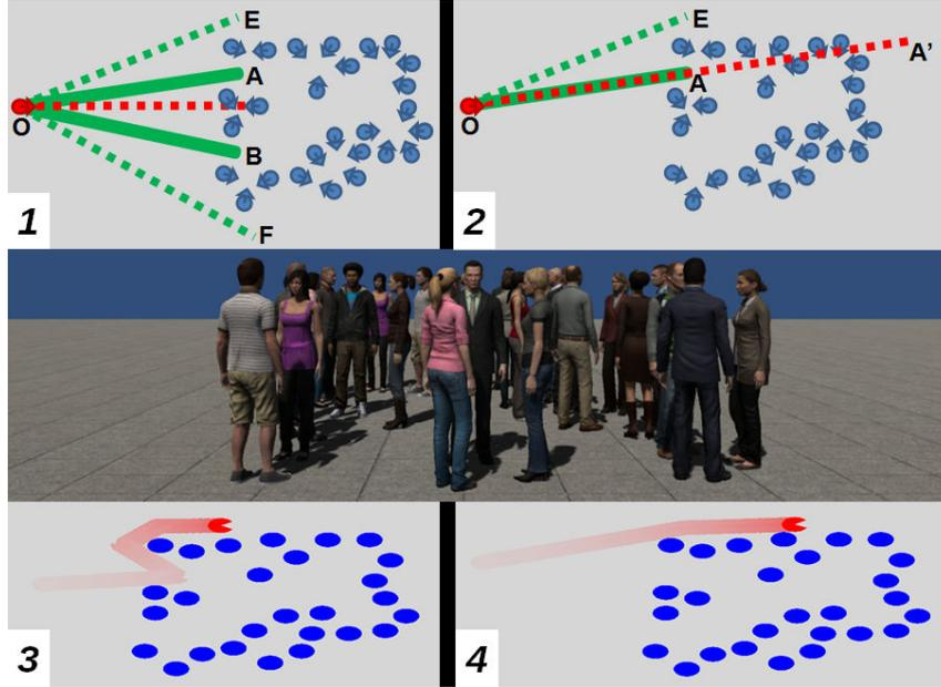
**Figure 4.8** 1) Without extra search, the algorithm stops at the IS  $OA$  and never considers  $OE$ . 2) With extra search, the IS  $OE$  is created by solving the collision on the IS  $OA'$ . 3) Agent's trajectories without extra search, the agent starts to go inside the crowd before backing up and going around. 4) With extra search, the agent is able to directly go around the crowd.
