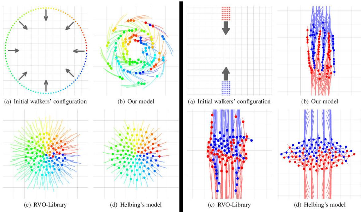
**Figure 2.14** Two typical situations used for visual evaluation. On the left, it is a circle with everyone trying to switch places with the one on the opposite side. On the right, it is two flows on a frontal collision course with each other. In both cases, we can see some models having difficulties to produce fluid movement that would look more natural. These comparisons are from [OPOD10] and the "our model" correspond to the vision based model.
