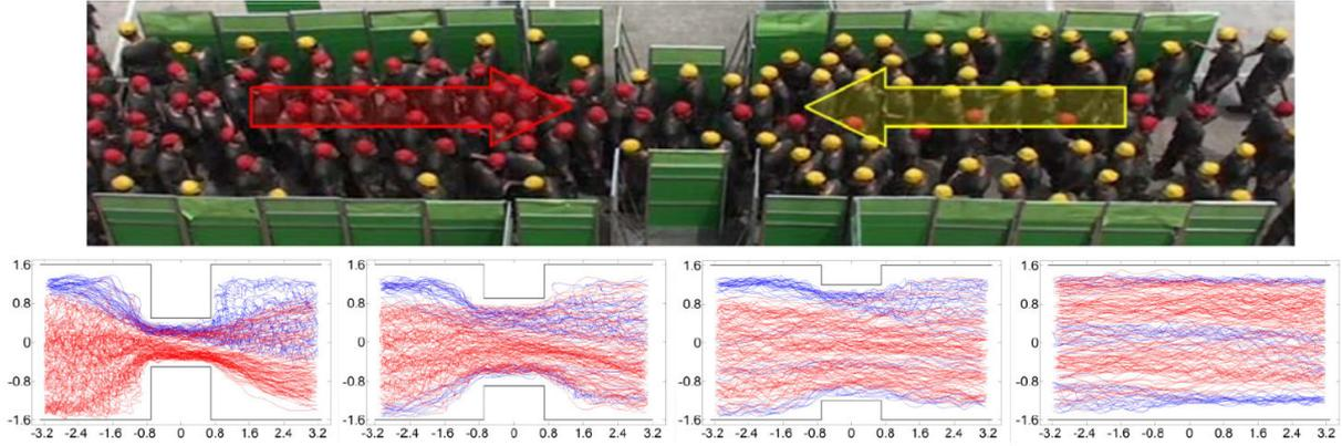
**Figure 2.13** Counter flow study from [DDH<sup>+</sup>14b]. Top: snapshot of the experiment. Bottom: Trajectories of pedestrians within the channel in each experiment scene.
