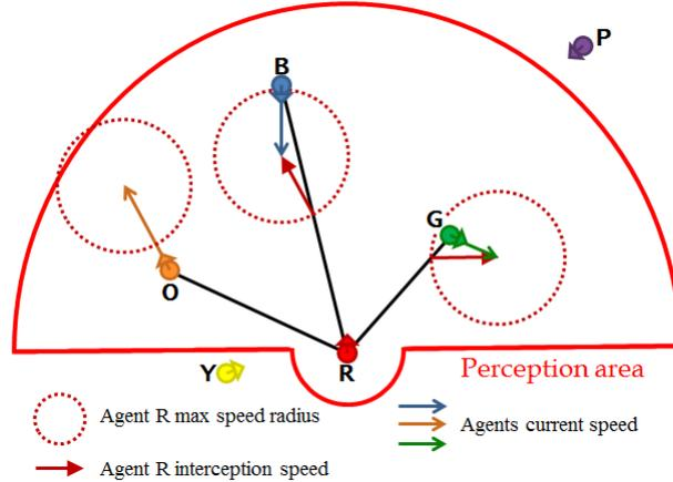
**Figure 4.6** Agent R perception system: First it selects the agents inside the perception area (O, B and G) then for each selected agent it computes the interception speed and selects the  $n$  agents with the smallest Minimum Interception Time (MIT) as neighbors (First B then G, O is not selected as it is going away too fast to be intercepted).
