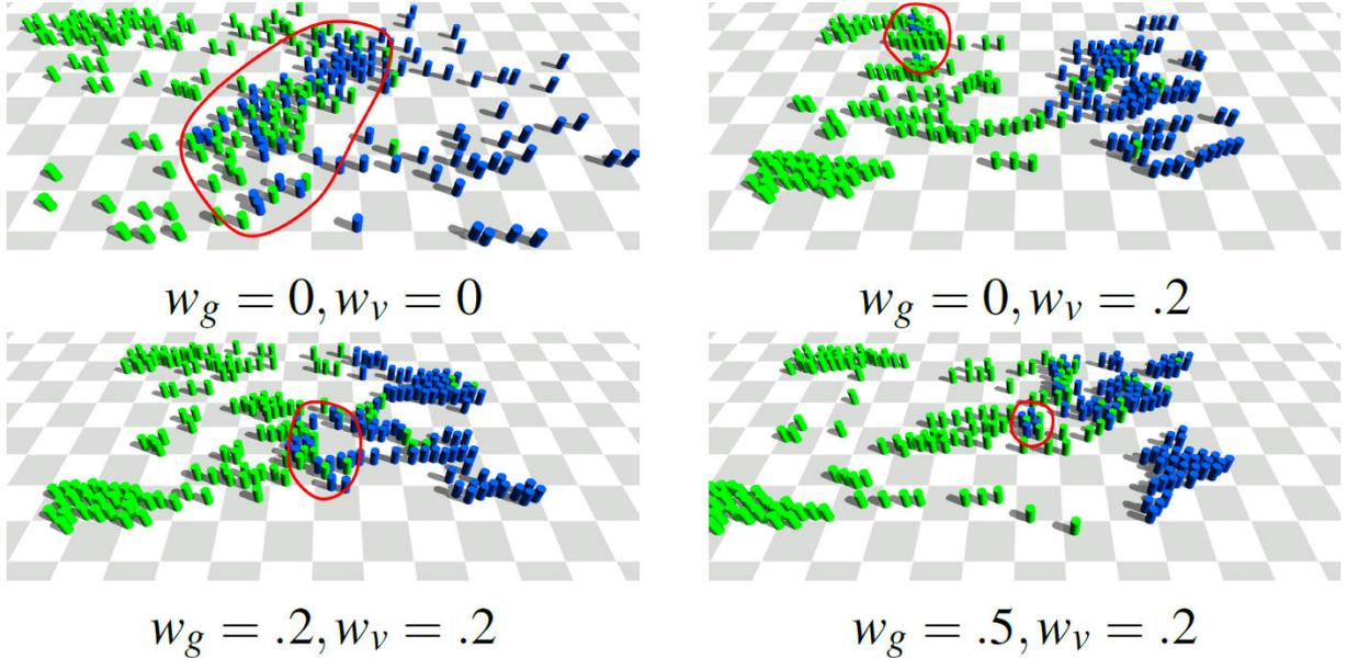
**Figure A.5** Simulations of a group (in blue) going through a crowd of individuals (in green) for different value of preference weights. The more the balance is in favor of grouping the tighter the group's clusters are. Moreover, with a balance in favor of grouping, no blue agent end up alone.
