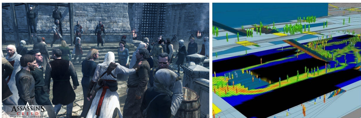
Figure 1.2 – Left: player interacting with a virtual crowd in the game Assassin's Creed. Right: Massmotion simulation result of the design for a new Transbay Terminal in San Francisco indicating that early designs of the terminal building contained problem areas from a pedestrian circulation point of view due to insufficient channel widths in what were predicted to be high volume routes.
