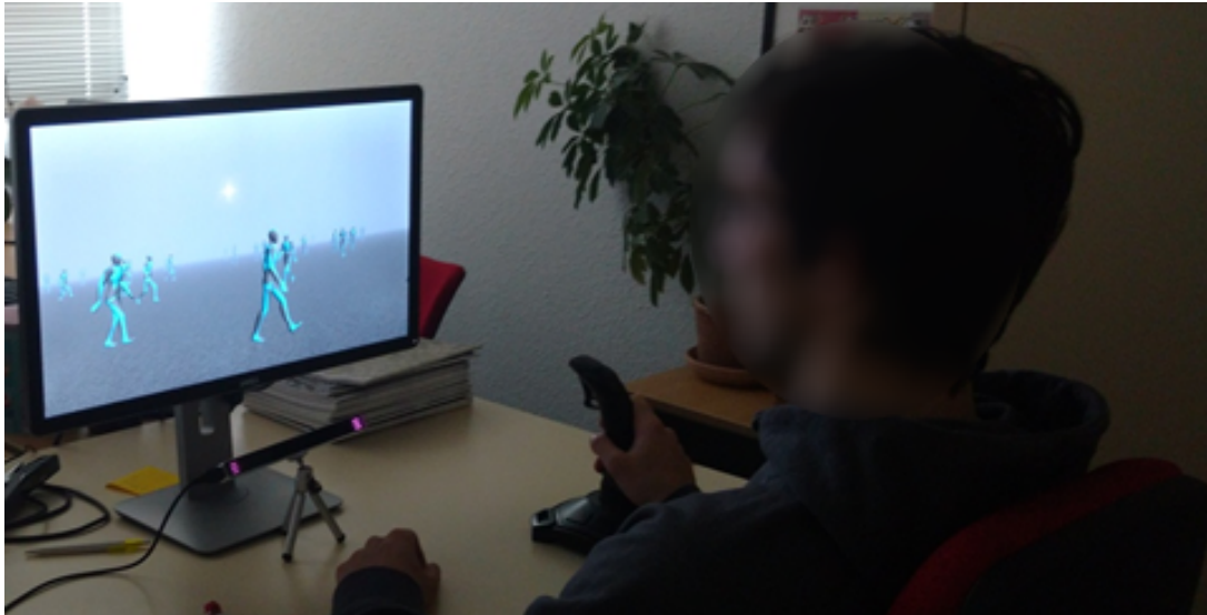
Figure 6.5 – Participant using the joystick to navigate in the virtual environment while his eyes are being tracked by the eye tracking device below the screen (the captor with purple dots on each side).
