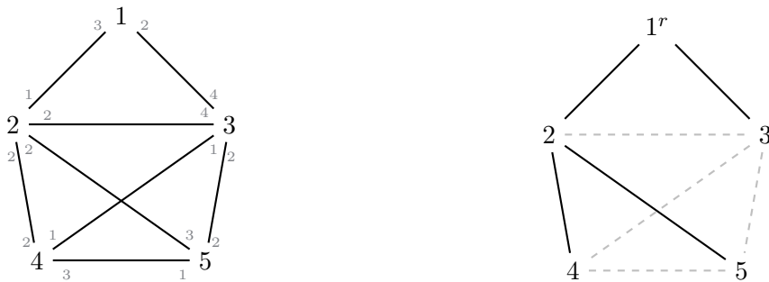
(a) Assignment of PortCosts (in gray) and BridgeIDs (same value as node id).
