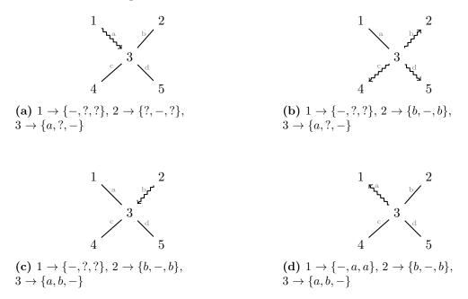
**Figure 1.1:** Example of transparent bridging. The caption of each subfigure represents the lookup tables of nodes 1 to 3, at each moment of the process. Notation e.g.  $1 \to \{-, x, z\}$  indicates that in order to send a message to node 2 and 3, node 1 must relay it through, respectively, segments x and z.
