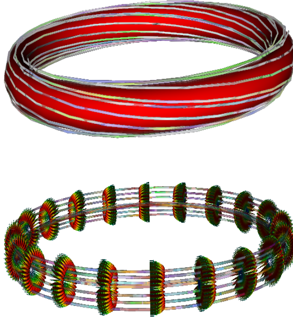
FIGURE 5.1: Initial data for 3D computation with the density and magnetic streamlines (top) and perturbation of the first Fourier mode of the velocity (bottom). The perturbation has an order of magnitude of 10^{-12} .
