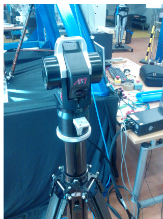
FIGURE 5.2 – Laser tracker, robot CoGiRo, Lirimm
