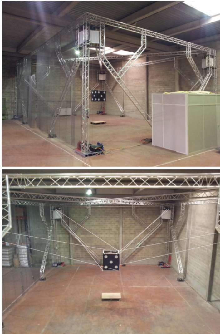
FIGURE 2.10 – CoGiRo : configuration suspendue
