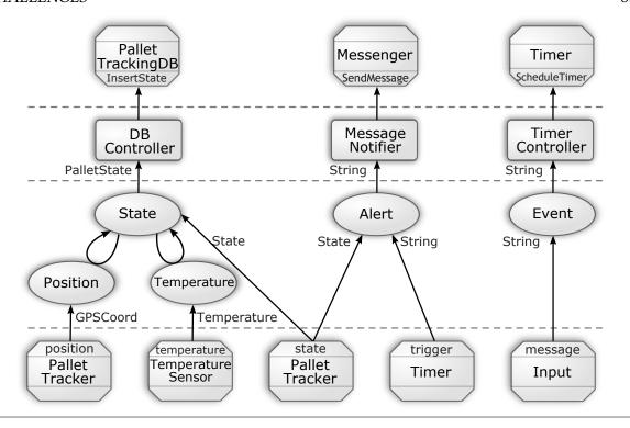
Figure 7.4 – The architecture of the PalletTracker application.
