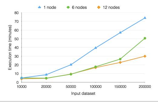
Figure 5.3 – Performance comparison between different cluster setups.
