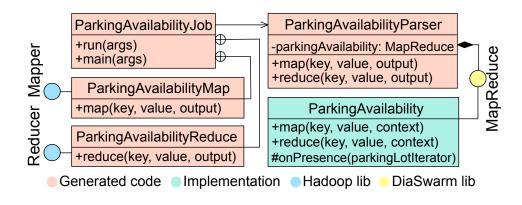
Figure 5.2 – The generated support for integrating Apache Hadoop.
