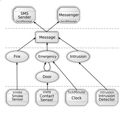
Figure 7.5 – The architecture of the HomeAlarm application.
