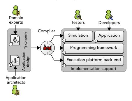
Figure 7.1 – DiaSuite tool support for the SCC application lifecycle.
