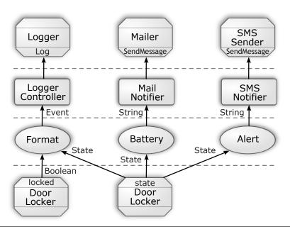
Figure 7.2 – The graphical view of the DoorLocks application.
