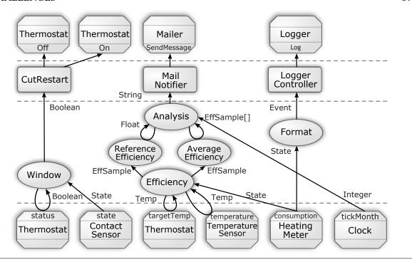
Figure 7.6 – The architecture of the HeatingMonitor application.
