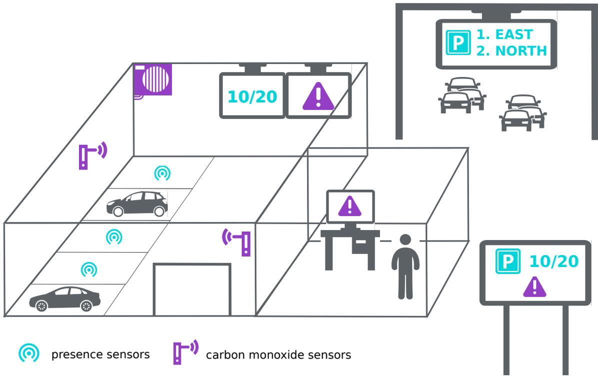
Figure 3.1 – A graphical representation of the parking management system.
