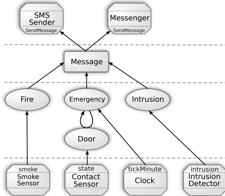
Figure 7.5 – The architecture of the HomeAlarm application.
