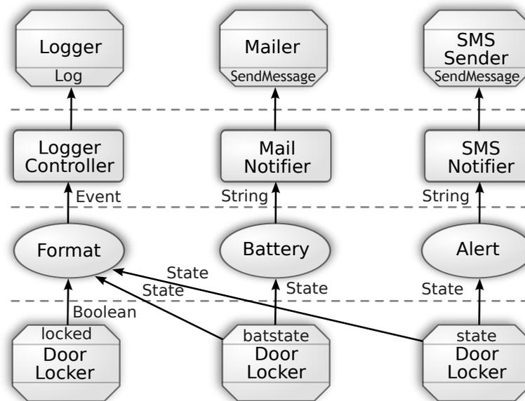
Figure 7.3 – The architecture of the DoorLocksPlus application.
