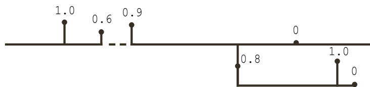
FIGURE 3.12: Staff representation of a group containing a dynamic delay and a sub-group.
