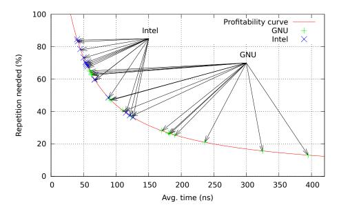
Figure 2.6: Profitability curve of memoizing transcendental functions
