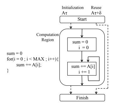
Figure 1.3: Scope of Region Based Memoization
