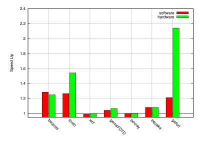
Figure 4.4: Speed-Up by Hardware Memoization for SPEC Benchmarks
