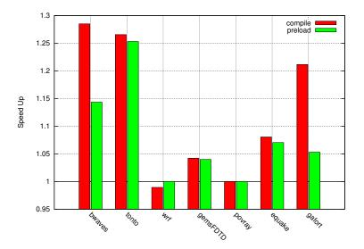
Figure 3.3: Speed-Up by Memoization for SPEC benchmarks 64k entry table, Intel Ivy bridge 2.3 GHz.
