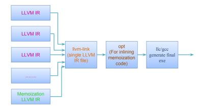
Figure 3.2: Flow Diagram of Memoization
