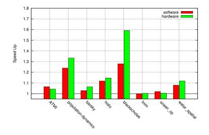
Figure 4.5: Speed-Up by Hardware Memoization for Selected Applications
