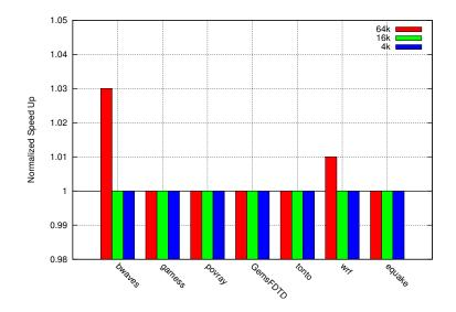
Figure 2.5: Memoization of SPEC benchmarks on Intel Ivy Bridge for different table sizes (icc)
