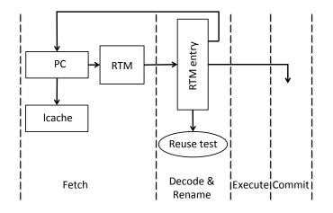
Figure 1.2: Implementation of Trace Level Memoization
