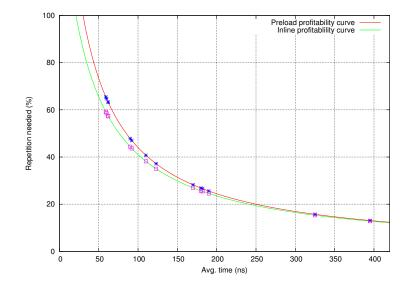
Figure 3.1: Profitability Curve - preload vs inline
