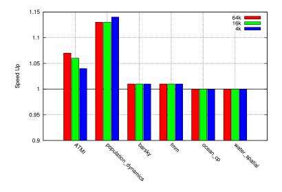
Figure 2.7: Memoization of selected applications on Intel Ivy Bridge for different table sizes (icc)
