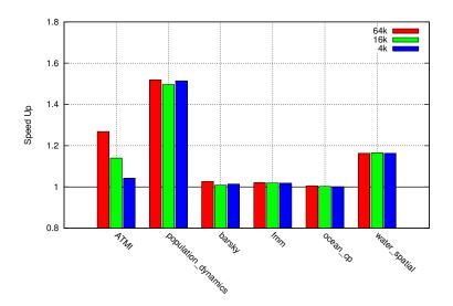
Figure 2.4: Memoization of selected applications on Intel Ivy Bridge (GNU compiler) for different table sizes
