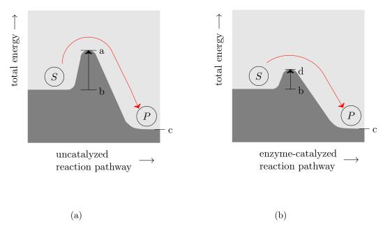
Figure 1.2: Activation energy. (a) The activation energy (energy a minus energy b) is required to transform S into P. (b) An enzyme lowers the activation energy (energy d minus energy b). The figure is adapted from Alberts et al. (2010).
