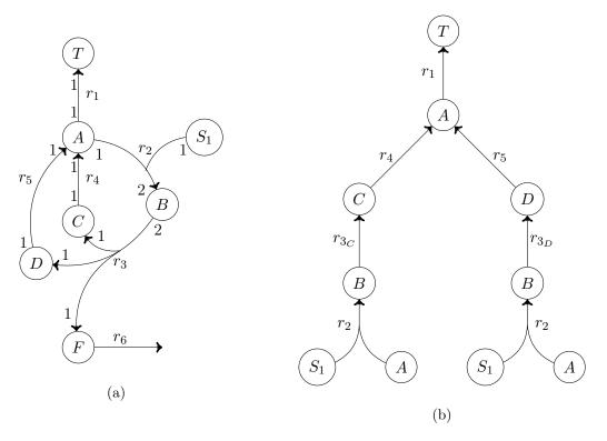
Figure 4.10: The toy network is depicted in 4.10a with the minimal stoichiometric precursor set  $S_1$  for the production of the target T. The recursion tree of the target and reaction decomposition steps in the many-to-one network is shown in 4.10b
