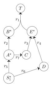
Figure 4.8: A metabolic network with several essential compounds (denoted by a \*). The reactions  $r_6$  and  $r_7$  do not take part of any minimal cut set of a subnetwork containing the reactions that respectively consume or produce a single essential compound. However,  $r_6$  and  $r_7$  build a minimal cut set for the factories from  $S_1$  to T.
