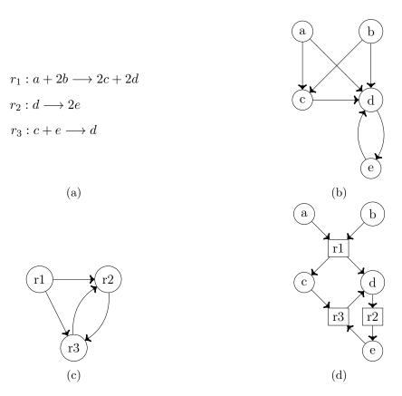
Figure 2.1: Metabolic network (a) modeled as a compound graph (b), reaction graph (c) or a bipartite graph (d).
