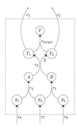
Figure 4.3: All compounds except T are considered as internal compounds. Here, the single steady state stoichiometric factory from  $X = \{S_1, S_2, S_3\}$  to  $\mathcal{T} = \{T\}$  contains all reactions except  $r_1$ , and coincides with the elementary mode that contains  $r_{target}$ . There is a second elementary mode that contains all reactions except  $r_{target}$ .
