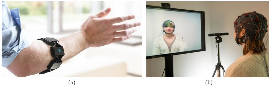
FIGURE 2.13 – Two examples of direct input devices. (a) The Myo armband acquires the forearm bioelectric signals in order to detect gestures and motions. (b) An example of EEG cap used for an AR application: the mind mirror [Mercier-Ganady et al., 2014] allows a user to see his brain activity.
