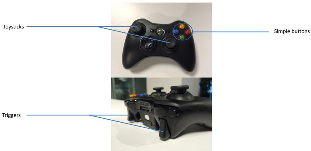
FIGURE 2.10 – The Xbox360<sup>TM</sup> gamepad is a classic game controller composed of joysticks, triggers and simple buttons. This kind of device is commonly used for playing video games.
