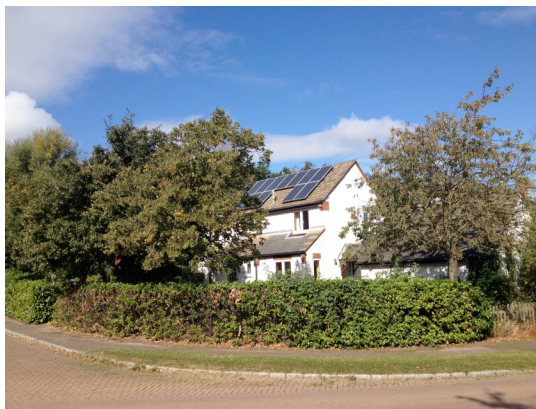
Figure 4-3 Estimating solar generation is not as easy as we could think (H2 WM ). Location, orientation, tilt, shading from trees, weather, etc. are many variables impacting on the generation
