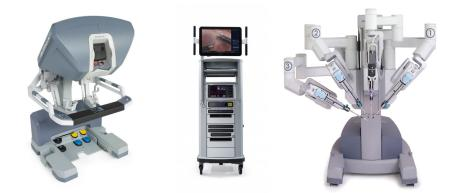
**Figure 6.2:** The *da Vinci*<sup>®</sup> robot. On the left is the surgeon console, in the center the vision cart, and on the left the robot itself.
