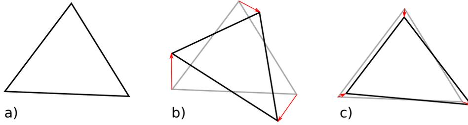
**Figure 3.3:** The co-rotational formulation allows to extend the validity of Hooke's law to large displacement if the strain is small. a) Initial shape of an element. b) The shape of the element after deformation. The initial shape is displayed in grey and the node displacement as red arrows. c) Deformed shape without the rotational component of the displacement.
