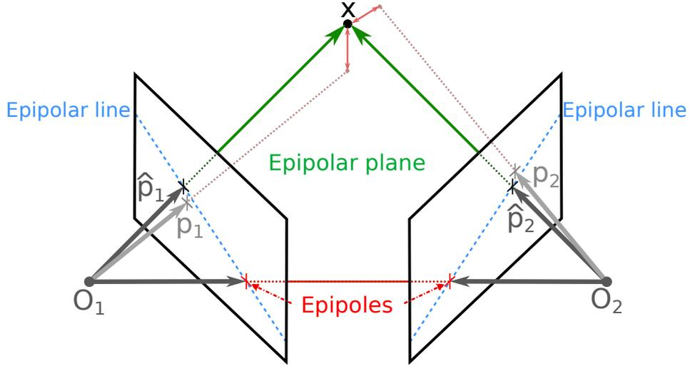
**Figure 1.14:** Triangulation. The dashed gray lines, in the direction of  $\mathbf{p}_1$  and  $\mathbf{p}_2$  are not secant. After the optimization algorithm the lines in the direction of  $\widehat{\mathbf{p}}_1$  and  $\widehat{\mathbf{p}}_2$  intersect at the point  $\mathbf{x}$ , the reconstructed position of the three dimensional point corresponding to the features  $p_1$  and  $p_2$ .
