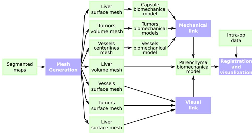
**Figure 3.4:** The liver surface is represented by two meshes: one for the visualization of the organ and the other for the mechanical model of the Glisson capsule. These two meshes can be the same or the visual mesh can be finer than the mechanical one.
