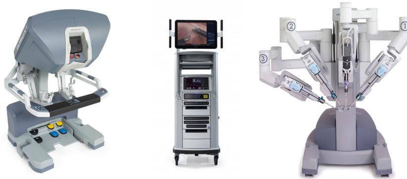
**Figure 6.2:** The *da Vinci*<sup>®</sup> robot. On the left is the surgeon console, in the center the vision cart, and on the left the robot itself.
