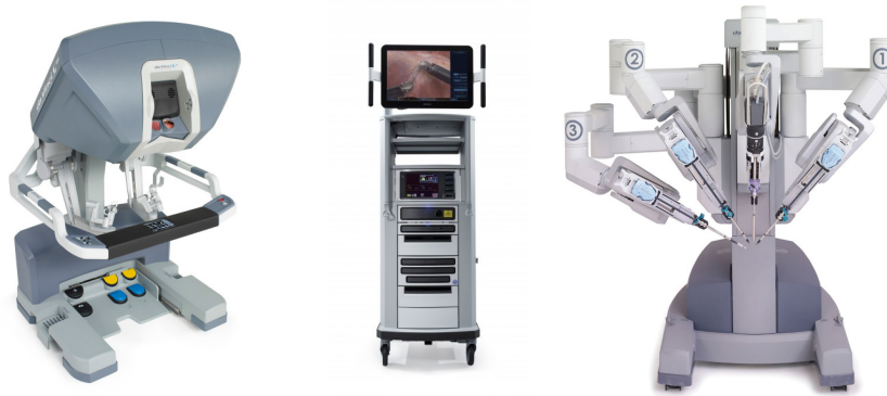
Figure 6.2: The da Vinci ® robot. On the left is the surgeon console, in the center the vision cart, and on the left the robot itself.
