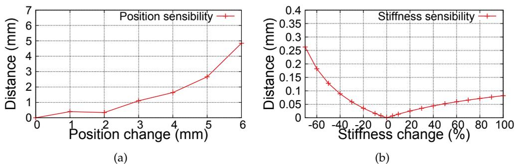
**Figure 5.11:** Sensitivity study. Mean Hausdorff distance between the final configurations of a reference model and a biomechanical model with altered boundary conditions position (a) and stiffness (b).
