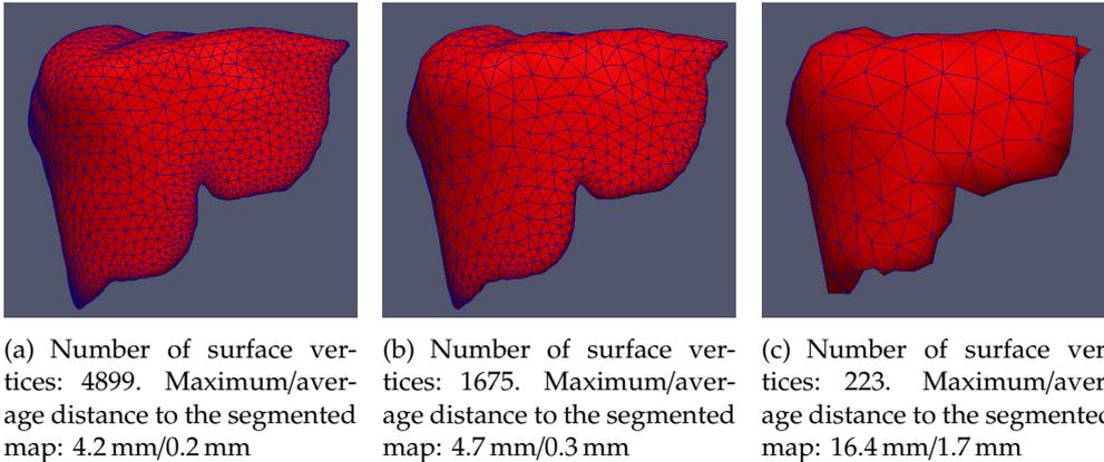
**Figure 1.9:** Errors induced by the mesh representation. The surface meshes were generated from the smoothed segmented map with the following parameters:  $\alpha = 30^\circ$ ,  $s = 30$ , and  $d = 0.5$  (a),  $d = 1$  (b),  $d = 5$  (c). Increasing the facet distance parameter reduce the number of vertices but increase the distance between the mesh and the segmented map.
