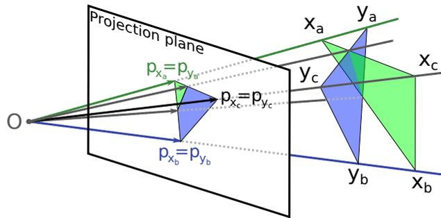
(b) Generation of a projective image.  $\mathbf{o}$  is the position of the camera. The  $\mathbf{p}$  are shown as arrows. This example is a special case: the projection of  $x_i$  and  $y_i$  for  $i \in \{a, b, c\}$  are the same. Adapted from Baecker.
