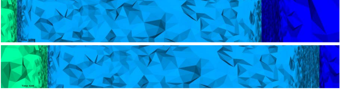
Figure 6.14: Zoom on the mesh and solution at the beginning (top) and at the end (bottom) of the last sub-interval. One can see the two waves move forward in the adapted bands.
