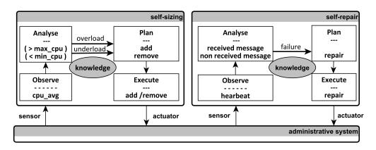
Figure 5.6 – (left) The architecture of the self-sizing manager, (right) the architecture of the self-repair manager
