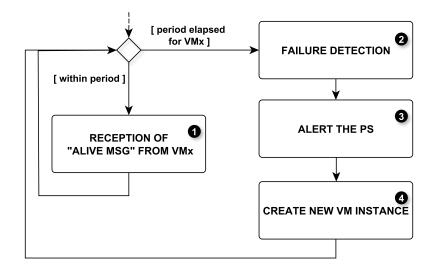
Figure 4.9 – The RM behavior when detecting a VM failure
