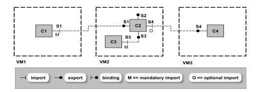
Figure 4.2 – Example of an application model (after binding ports)
