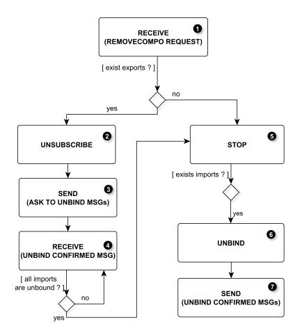
Figure 4.7 – The agent behavior when removing a component
