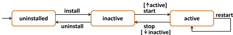
Figure 3.1 – An example of a state machine associated to a resource driver
