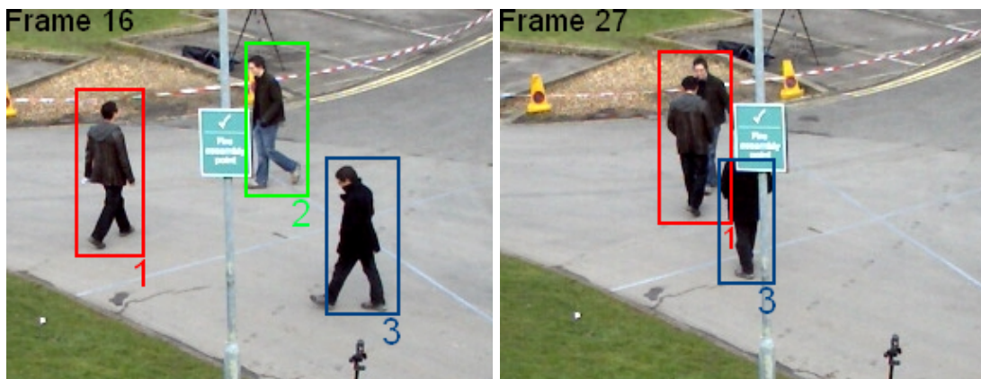
Figure 2.6: Easily found error due to occlusion
