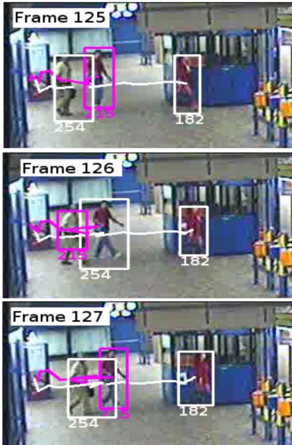
Figure 4.10: Illustration of the output of the controlled tracking process. Different IDs represent different tracked objects.
