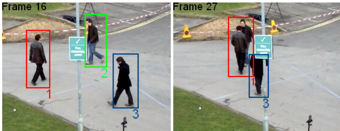
Figure 2.6: Easily found error due to occlusion
