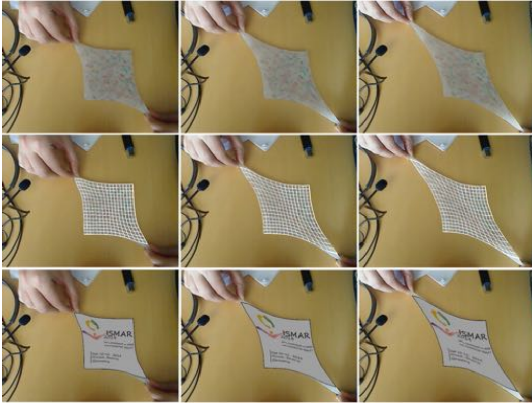
Figure 3.6: Selected frames during a 2D elastic surface augmentation of the silicone-like material when being stretched up to 120%, with (top) input images (middle) registered mesh (bottom) surface retexturing.
