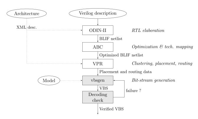
Figure 3-7 – The Virtual Bit-Stream design flow, based on the Verilog-To-Routing framework. The Virtual Bit-Stream design flow relies on the Verilog-To-Routing framework to generate placement and routing data. The vbsgen back-end is subsequently used to generate custom bit-streams using a custom model. A decoding step is added after the bit-stream generation to ensure that the Virtual Bit-Streams created will be decodable at runtime, and to regenerate non-compliant bit-streams.
