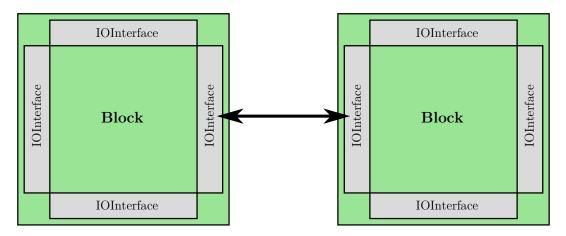
Figure 3-10 – Block model used in the vbsgen framework. Each element of the model array derives from the root type Block of the vbsgen framework. A Block contains IOInterfaces on all of its four sides. These interfaces model the connection points between the block and its neighbors and serve to determine the relationships between elements of the model array during the bit-stream generation.
