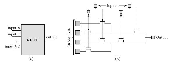
Figure 1-4 – Architecture of a 2-LUT using memory cells and passtransistors. In an SRAM FPGA device, the most convenient way of implementing multiplexers is to use pass-transistors. The implementation of a k-LUT requires  $2^k$  memory cells and a k-to-1 multiplexer, here implemented using a tree of passtransistors, although more optimized versions are more commonly used.
