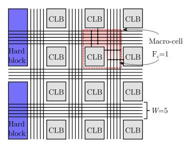
Figure 3-2 – Example of an island-style architecture and its repeatable *macro-cell*. The considered architecture is a generalized island-style logic array and its mesh routing network. Ignoring localized heterogeneity, a repeatable pattern can be identified, duplicated in both directions, which is what we consider in this document as a macro-cell.
