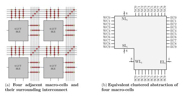
Figure 3-6 – Clustering multiple macro-cells together before coding the Virtual Bit-Stream. Using the Virtual Bit-Stream technique, it is possible to use a coarser level of abstraction by grouping multiple macro-cells together prior to the calculation of the route list. The clustering offers the possibility to represent the routes with even fewer data, but at the cost of more complex decoding operations.
