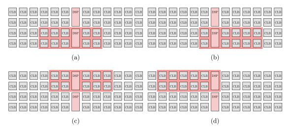
Figure 5-4 – Multiple relocation possibilities for the same bit-stream of a task. As the connections between the homogeneous routing and the hard blocks can be made at multiple equivalent points of connection within switches, the task benefits from an increased flexibility in its horizontal placement. The vertical placement possibilities are still limited by the common denominator of the hard blocks heights.
