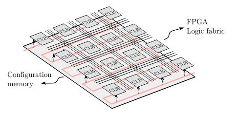
$\label{eq:Figure 0-11} Figure \ 0\mbox{-}11\ -\ {\bf Overview} \ \ {\bf of} \ \ {\bf an} \ \ {\bf FPGA} \ \ {\bf architecture} \ \ {\bf and} \ \ {\bf its} \ \ {\bf configuration} \ {\bf mechanism}$
