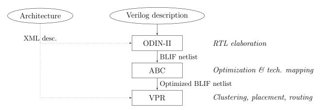
Figure 2-5 – The Verilog to Routing design flow
