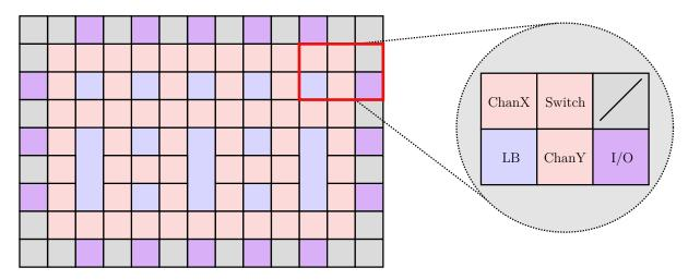
Figure 3-9 – **The** *vbsgen* **model array.** *The internal model of an architecture in* vbsgen is a two dimensional array where each element represents one basic feature *of the FPGA: soft logic, routing, input/outputs, etc. Each block relies on a special*-*ization of classes of the model framework. Once built, the model array is populated using placement and routing data, and eventually dumped as a bit-stream.*
