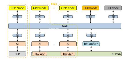
Figure 7-2 – Overview of the FlexTiles platform heterogeneous many-core hardware architecture [Jan+15].
