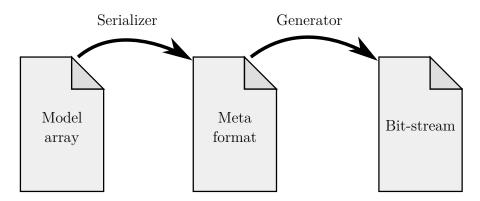
Figure 3-11 – Generation of intermediate representations and final bitstream in the vbsgen framework. From the designer perspective, the usersupplied vbsgen model fills a meta-structure dedicated to a specific output format (e.g. virtual or conventional bit-stream) instead of actually creating binary structures, using a user-defined Serializer. The conversion process from the metastructure to the final bit-stream is ensured by a Generator included in the framework.
