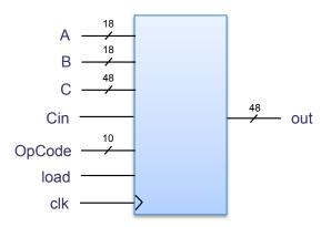
Figure A-6 – Arithmetic accelerator (DSP block) overview
