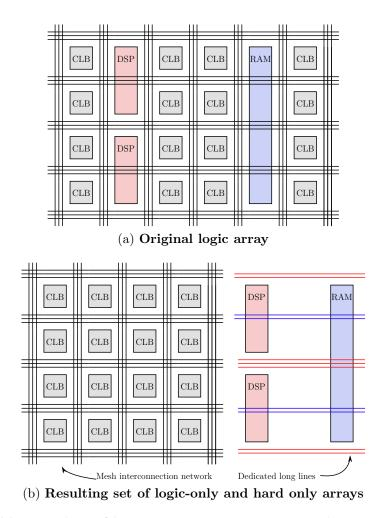
Figure 5-2 – Abstraction of heterogeneous resources. The original logic array, based on an island-style architecture, contains CLBs as soft logic elements and two types of hard blocks. The interconnection network is shared by both soft and hard blocks. In the abstraction of the logic array, the soft logic lies in one mesh interconnect network dissociated from the hard block routing. The connection to and from hard blocks is made via long lines dedicated to each type of hard block.
