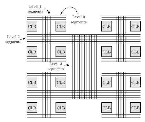
Figure 1-12 – **Overview of a hierarchical interconnect architecture.** In a hierarchical architecture, the routing network is split in multiple levels in the same manner as an H-tree. The delay model is simpler in this case since it can be finely estimated from the global routing, given the number of interconnection levels crossed on a net path.
