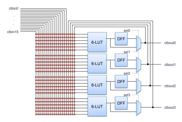
Figure A-4 – Details of a Complex Logic Block (CLB)
