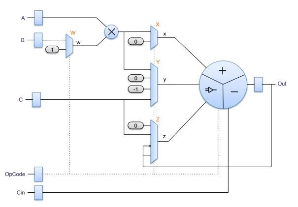
Figure A-7 – Details of an arithmetic accelerator
