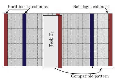
Figure 2-1 – Compatible patterns on a logic fabric for task relocation. The geometry of task  $T_i$  as well as the order of soft logic and hard block columns composing it must be preserved to allow for its relocation. Considering these constraints, the technique in [Kra+06] can only relocate  $T_i$  to the rightmost position.
