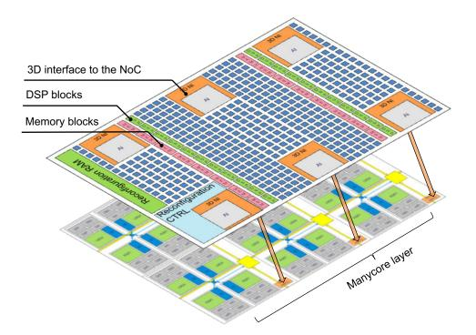
FIGURE 0-10 – La plateforme 3-D FlexTiles.
