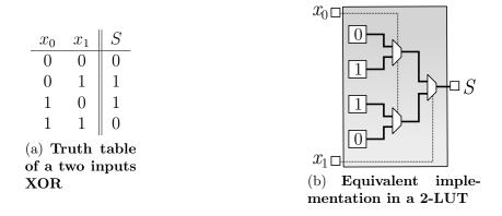
Figure 1-2 – Implementation of a two input boolean equation in a Look-Up Table. The 2-LUT can be seen as a small memory whose address lines are in fact the boolean equation inputs. Given the inputs  $(x_0, x_1)$ , the cascading multiplexers of the memory will output one of the memory cell logic value, which have been configured beforehand to store the logic function  $S = x_0 \oplus x_1$ .
