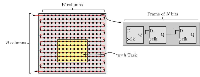
Figure 6-6 – Basic organization of a standard of hybrid scan-path over the programmable device. The static scan-path traverses the configuration memory in a serpentine way, line by line. The considered smallest units of configuration are frames of N configuration bits.
