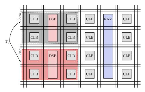
Figure 5-1 – Relocation problem in modern FPGAs. Task  $T_1$ , placed on a set  $S_{src}$  of resources, is only movable to another set  $S_{new}$  with resource types and positions matching those in the original set. The necessity to find matching partitions to perform the relocation of a task hampers the overall placement flexibility of the device.
