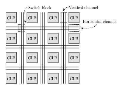
Figure 1-13 – Overview of an island-style interconnect architecture. Islandstyle architectures have regular logic fabric and routing interconnect. The routing network is split in vertical and horizontal channels. Switch blocks allow interconnecting the channels at their intersections.
