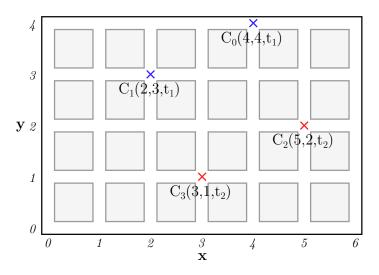
Figure 5-5 – Model of a task with abstracted heterogeneous hard blocks. Tasks are defined as a set of homogeneous logic elements and a variable number of connections  $C_i$  to hard blocks. Each connection  $C_i$  has to be linked to a hard block via heterogeneous-only routing. A valid placement of a task needs to satisfy the connection type constraint for all the connections.
