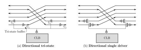
Figure 7-6 – Uni-directional routing in modern architectures.
