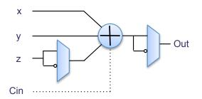
$\label{eq:Figure A-8-Details of the Arithmetic and Logic Unit} Figure A-8-Details of the Arithmetic and Logic Unit$
