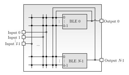
Figure 1-6 – Overview of a complex logic block. The complex logic block contains a cluster of N basic logic blocks containing k-LUTs whose inputs and outputs are connected to a crossbar interconnection network local to the CLB. I inputs are routed from the global interconnection network to the local crossbar, with I carefully explored to balance the area and logic occupancy of the logic fabric. All the N outputs of the basic logic blocks are routed to the global interconnection network.
