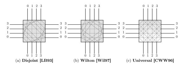
Figure 1-14 – Switch block topologies. Various switch block topologies have been explored, the disjoint, Wilton and universal models are three possible switch block implementations. While the disjoint topology may simplify the global-to-detailed routing step of the CAD flow, the Wilton topology shows an increased flexibility which can lead to fewer tracks used. The universal model meets the dimensional constraint but fails to be easily expendable to segmented routing schemes.
