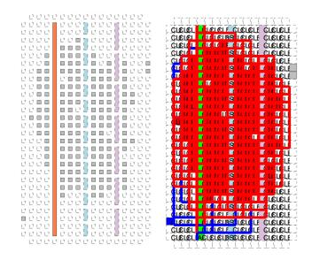
Figure B-2 – Placement and routing of the mult16x16 task
