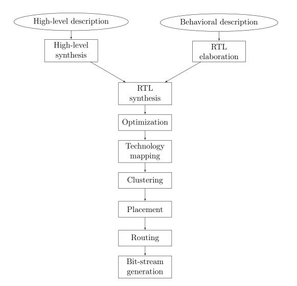
Figure 2-3 – A typical FPGA design flow
