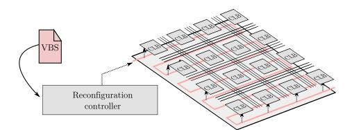
Figure 3-1 – Overview of the Virtual Bit-Stream technique integrated to a FPGA logic fabric. The Virtual Bit-Streams are decoded by a dedicated reconfiguration controller which decodes the alternate representation and loads it into the target logic fabric configuration memory.
