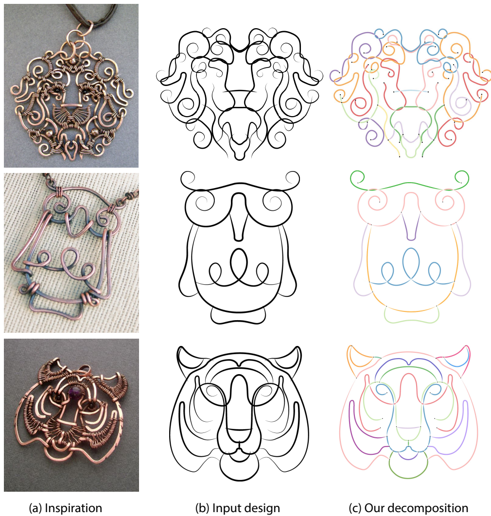
Figure 3.5: We use existing jewelry (a) as inspiration to test our algorithm. Given a bitmap drawing of the wire-wrapped jewelry (b), our solution (c) closely matches the original decomposition. The decompositions are identical for the lion and the owl, while the left ear of the tiger results in a slightly different configuration than the original, although with the same number of wires.
