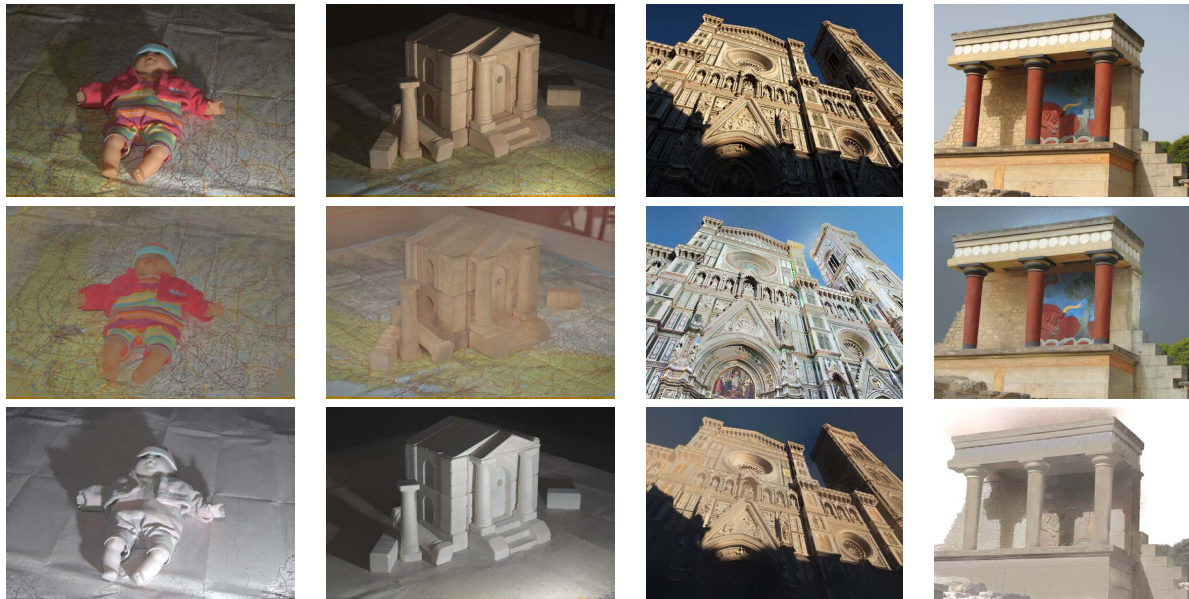
Figure 3.6: Our extracted layers on captured (left) and internet photographs (right). In each case, the first row contains the input image, the second row is the reflectance and the third row is the illumination. (Laffont et al. 2012)
