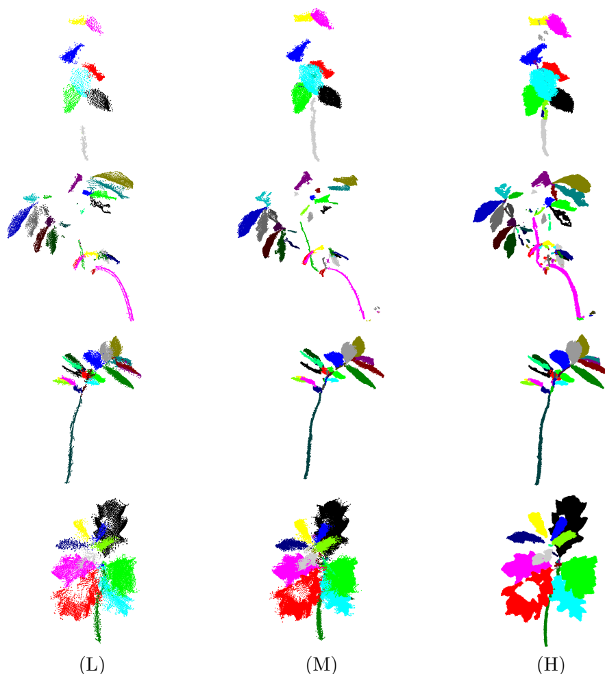
Figure 10. Segmentation results for point clouds of four contrasting plant seedlings with three different TLS resolution levels each. From top to bottom: birch, horse chestnut, sweet chestnut and red oak. On each point cloud, all points with the same colour belong to the same cluster.
