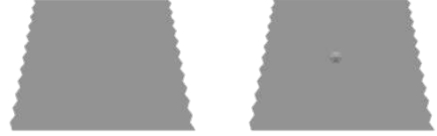
Fig. 4. Visual stimulus to measure the contrast sensitivity. Left: the reference plane. Right: a regular plane where a vertex is displaced.
