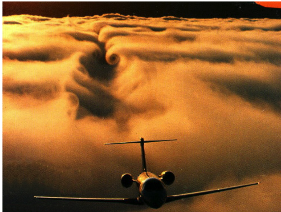
(a) Vorticity in the wake region ( Photo courtesy of Cessna Aircraft Company ).
