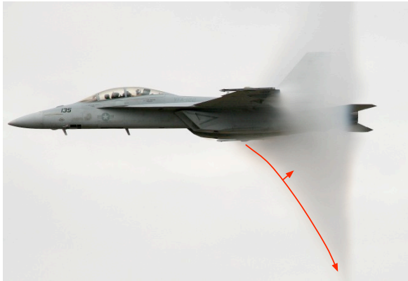
(a) Mach cone around a F-15. In red: the directions of anisotropy of the shock wave.
