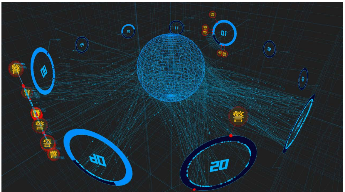
Figure 2.16: DAEDALUS [35] is a uses three dimensional visualisation. The centre of the view is occupied by a sphere divided into 256 by 256 points and capable of representing mapping an entire /16 network. From this sphere, emanating lines represent connections and points travelling along them are events. The sphere is surrounded by ring charts which each represent a monitored organisation with occupied address spaces and dark net spaces. Alarms triggered by these events are made visible using the Chinese character meaning “caution”.
