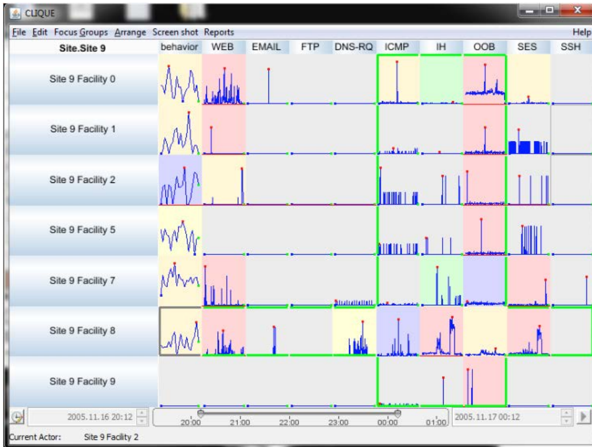
Figure 2.12: Based on LiveRac 6 , CLIQUE [14] offers a tabular organisation of data with columns for each service and rows for users. Each cell initially contains a sparkline type visualisation which can be expanded to show more detail.
