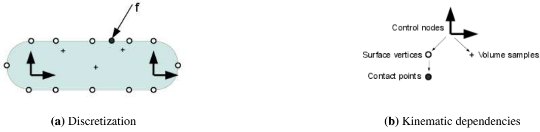
FIGURE 4.2 – Structure of a traditional model. Control nodes (here, moving frames), control surface vertices (empty circles) and volume sampling points (crosses). Contact forces are applied to surface points (filled circles) controlled by the surface vertices. (4.2a) : Discretization with control nodes and sampling points. (4.2b) : Kinematic dependencies.
