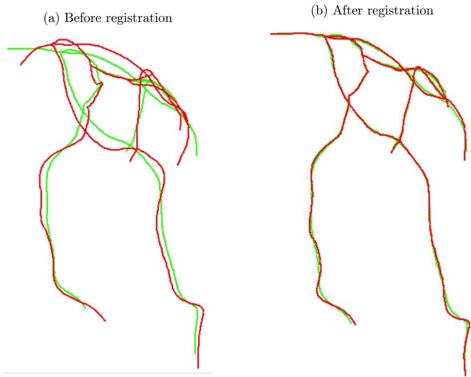
Figure 9.5: Preliminary results on non-rigid registration. (a) Deformed synthetic case defined as target (green) and the initial structure (red). (b) Non-rigid registered transformation of the initial structure (red) aligned with target (green) using non-rigid implementation of the TP-ICC algorithm.
