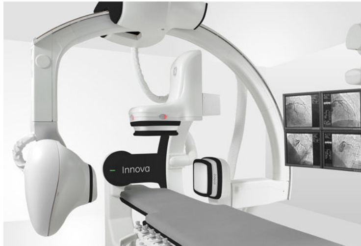
Figure 2.13: Example of bi-plane system: Innova IGS 630 from GE Healthcare. The secondary plane acquisition is provided by a ceiling mounted system.
