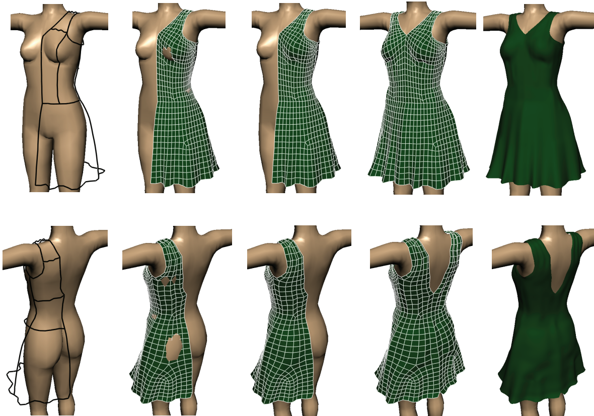
FIGURE 3.1 – The garment design process: sketch lines around the mannequin, quad-mesh the resulting network of lines, refit to underlying body, and produce the final garment by mirror and join operations.
