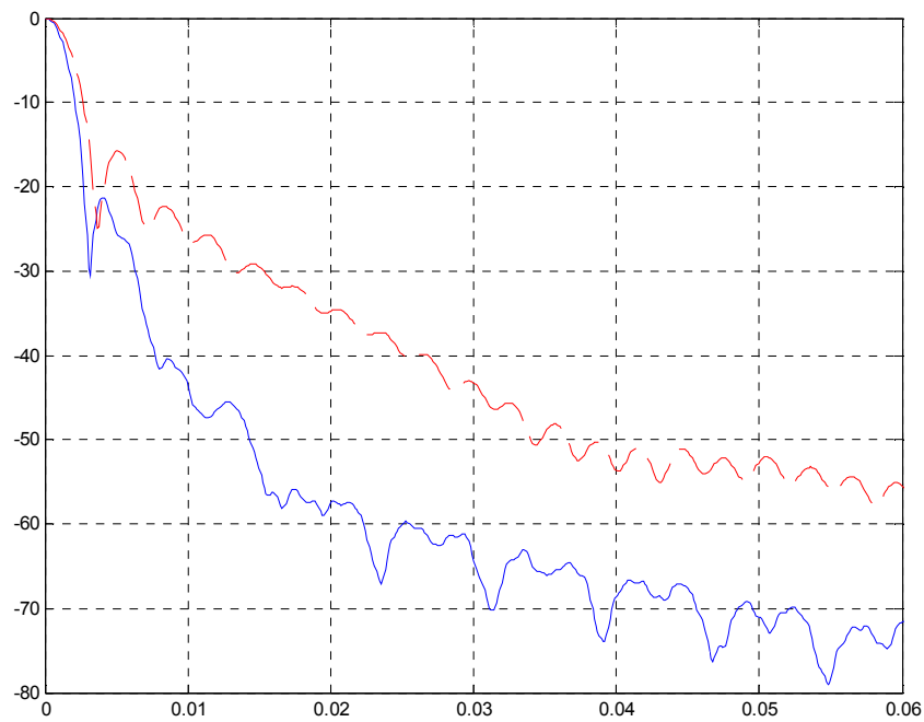
Figure 81 – ELD-AAC prototype (blue), LONG_START synthesis window (red)
