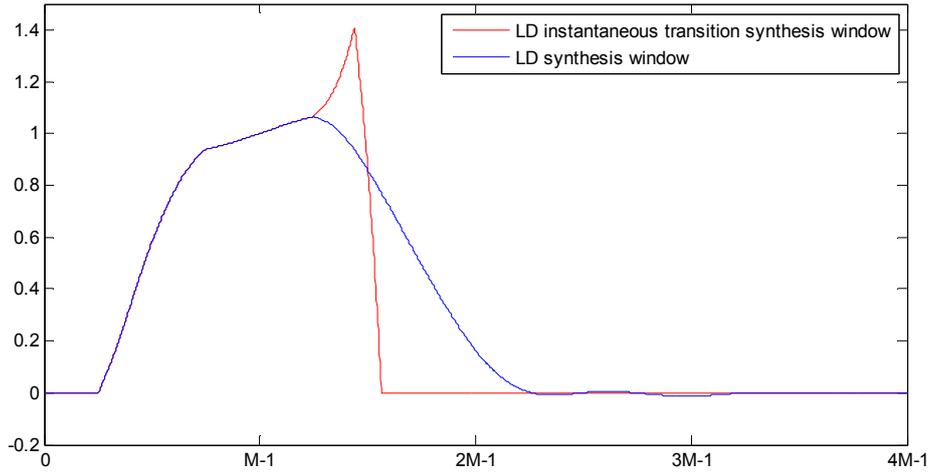
Figure 43 – Long synthesis window in normal operation (blue) and in case of low delay block switching  $w_1$  (red).
