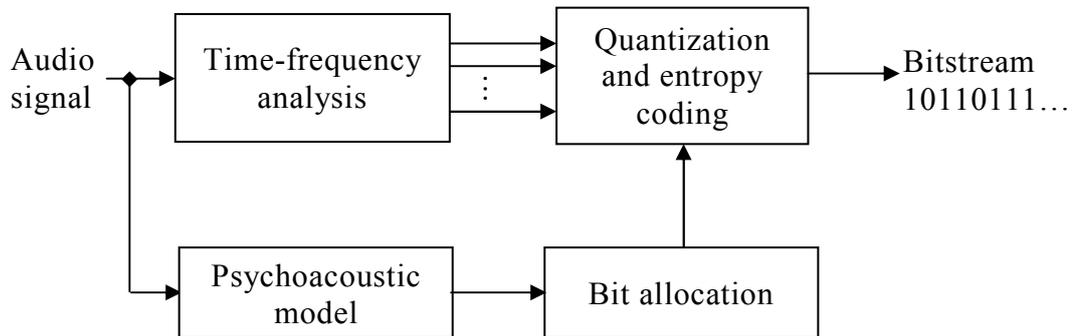
Figure 6 – General structure of a perceptual audio encoder
