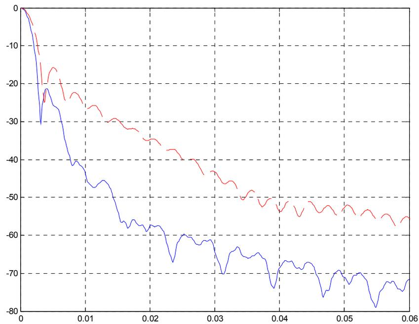
Figure 81 – ELD-AAC prototype (blue), LONG\_START synthesis window (red)
