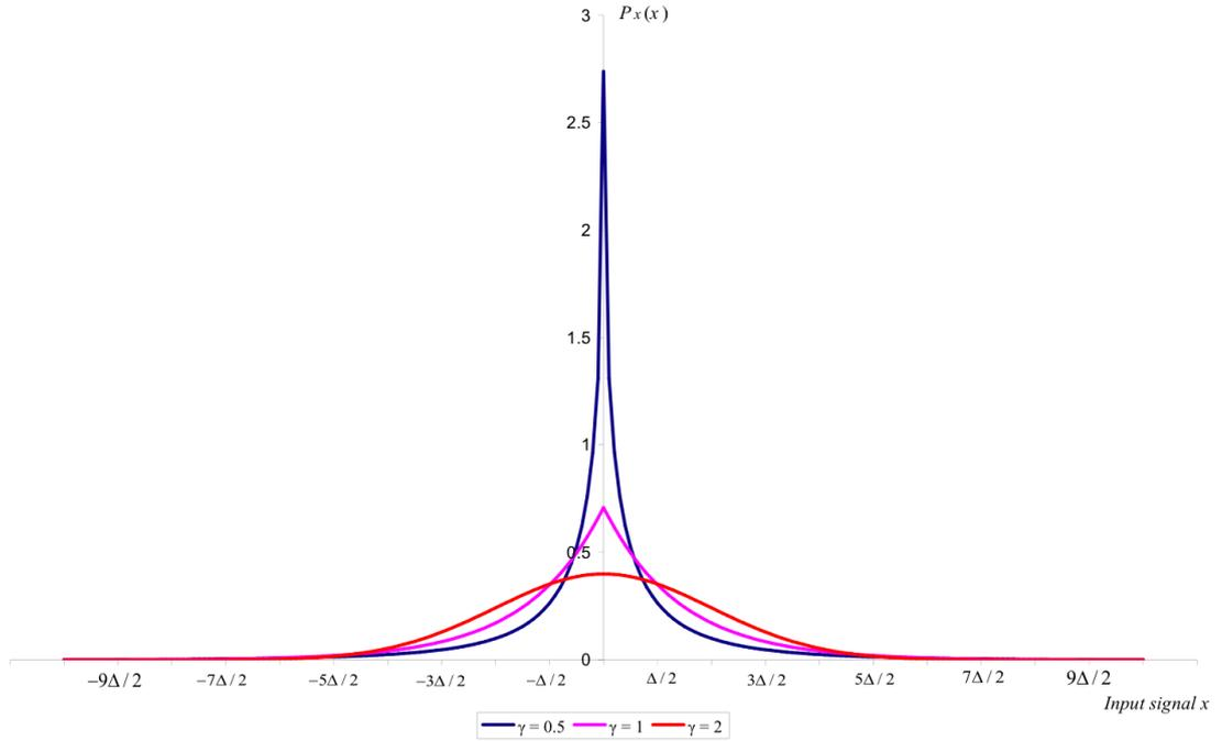
Figure 92 – Generalized Gaussian probability density function  $P_x(x)$
