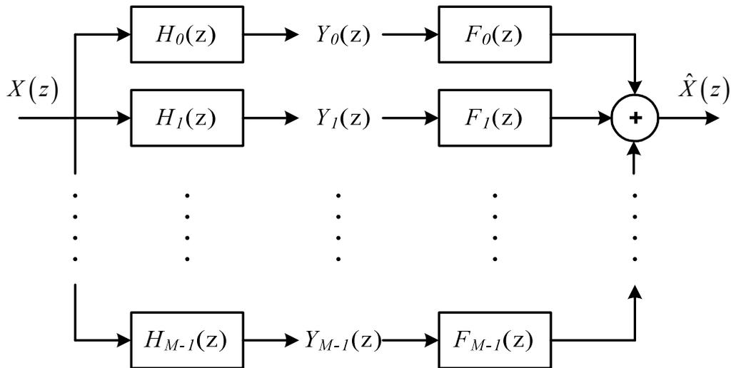
Figure 3 – Structure of filter bank with  $M$  sub-bands
