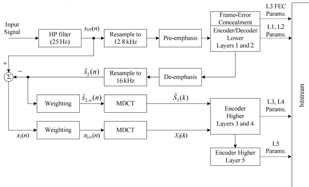
Figure 74 – Block diagram of the G.718 encoder
