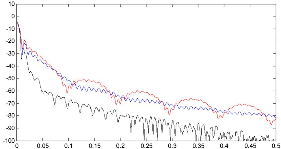
Figure 46 – Frequency responses (between 0 and 0.5) of low delay window (in black) low delay synthesis window for normal transition between low delay and short sine window (in blue) and low delay block switching synthesis window (in red)
