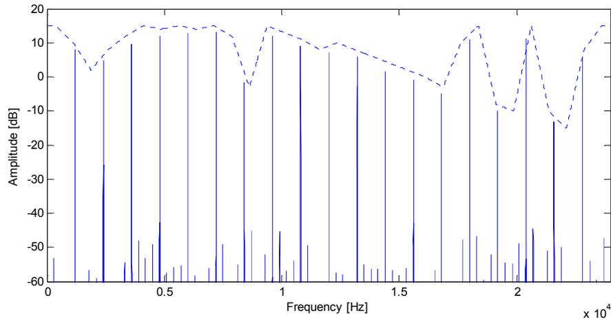
Figure 22 – Equalization using complex-exponential modulated filter bank
