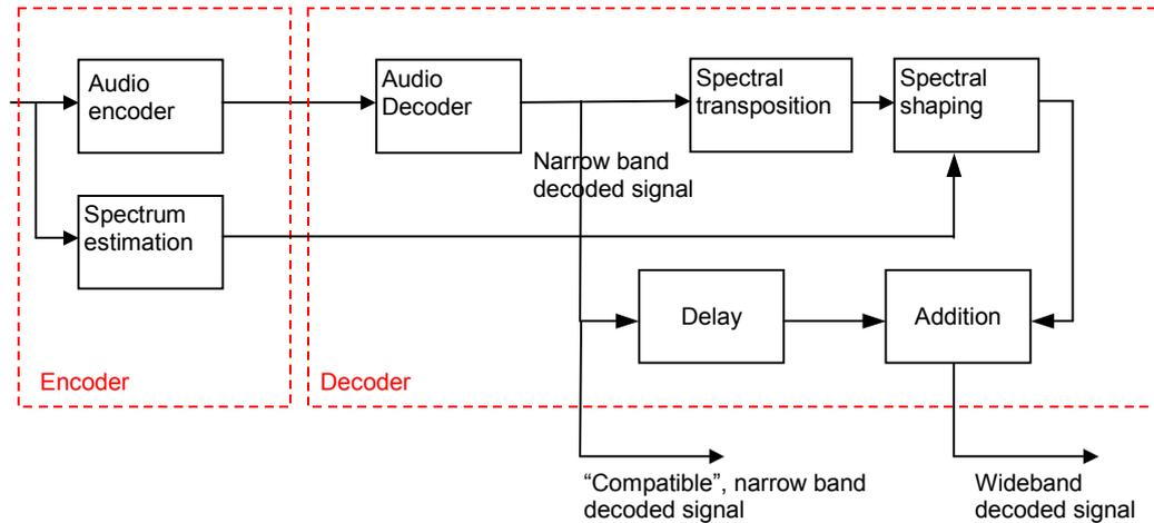
Figure 16 – Principle of the PAT codec
