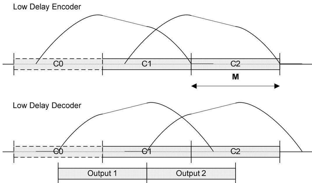
Figure 75 – Encoding and decoding timing with ALD window
