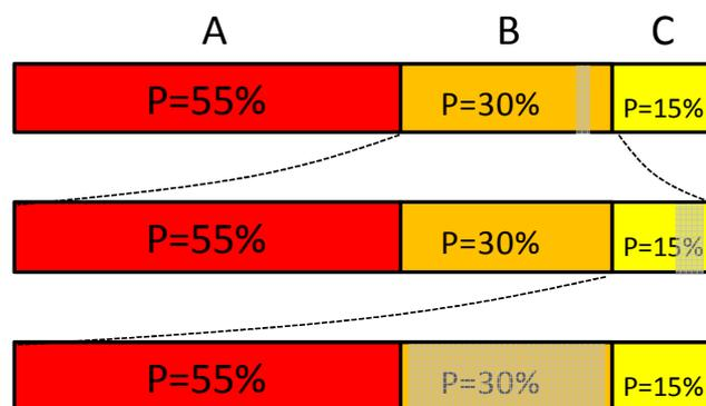
Figure 15 – Arithmetic coding (B-C-B are emitted)
