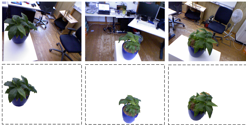
FIGURE 3.1: The multi-view segmentation problem: Given a set of input images of a scene, we want to identify and segment the object(s) entirely seen by all the cameras. In this case, it is the plant.
