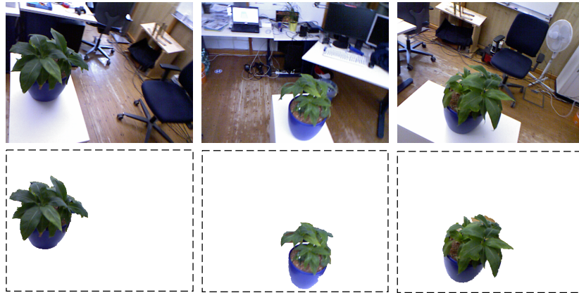
FIGURE 5.1: Multi-view object segmentation (MVOS) using our method with the 3 wide-baseline views shown only, with no photo-consistency hypothesis and no user interaction.
