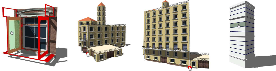
Figure 2.14: Interactive modeling of a building grammar. With an approach similar to classical 3D modeling software, the user can interactively set grammar rules during an editing process [LWW08].
