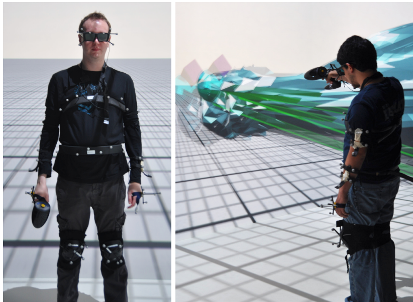
Figure 3.13 – Setup of our experiment. A subject with 11 position trackers used to record his posture and a Flystick to manipulate the objects (left), and a manipulation scenario of the 7-Handle technique in an immersive virtual environment (right).
