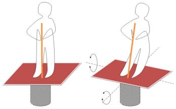
**Figure 8.1** – Principle of the Joyman interface for walking into virtual worlds. Following the example of joystick and standing on an articulated platform, users indicates their desired walking direction by leaning.
