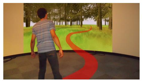
**Figure 10.4** – Illustration of the Shake-Your-Head technique with a slalom navigation in a virtual environment.
