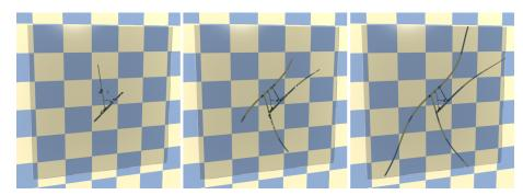
Figure 2.1 – Illustration of the energy-based criterion to stop the crack propagation using three glass slabs broken with different fracture toughness (the fracture paths have been highlighted during the rendering). The left slab has a toughness of  $150 \text{ J.m}^{-2}$ , the middle slab has a toughness of  $90 \text{ J.m}^{-2}$ , while the right slab has a toughness of  $60 \text{ J.m}^{-2}$ .
