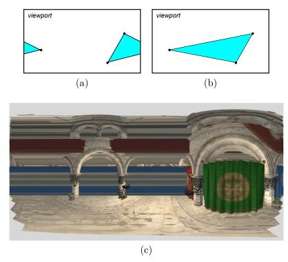
**Figure 5.5** — Rasterization of a triangle projected from rear fails when using an equirect-angular projection. Surface (a) is desired but (b) is generated. (c): the problem on a real scene: triangles composing the red an blue drape on the very right are rasterized across the whole viewport.
