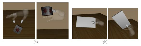
Figure 3.11 – (a) Grasping a cube from the edges with our approach: (left) uniform pressure distribution is not sufficient to lift the object, (right) non-uniform pressure distribution allows grasping. (b) Example of Coulomb-Contensou friction with our approach based on volume contact constraints. The fingers resist to moments around the grasping axis, and allow to rotate objects around that axis.
