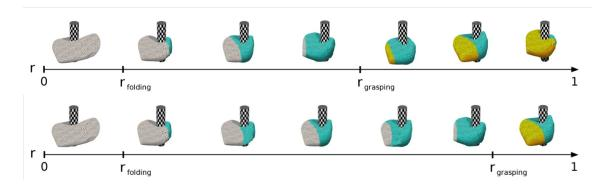
**Figure 9.3** – Our pseudo-haptic approach with the evolution of the grip force when grasping a virtual cylinder. The  $r_{folding}$  threshold is fixed while the  $r_{grasping}$  threshold varies in order to accommodate our pseudo-haptic effect. A progressive visual feedback composed of different colors informs the user about the different thresholds.
