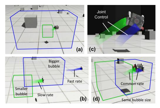
**Figure 9.6** — Illustration of the joint control technique. (a) Carrying an object without joint control; case where the smaller bubble (left) is in rate control and not the bigger bubble (right). (b) Difference in bubble size and workspace translation speed without joint control. (c-d) Carrying an object with joint control.
