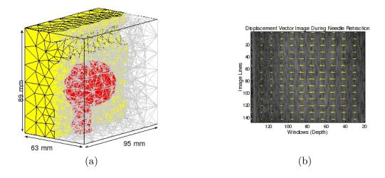
Figure 3.3 - (a) Tissue phantom meshed with tetrahedral elements and (b) estimation of tissue displacements using elastography.
