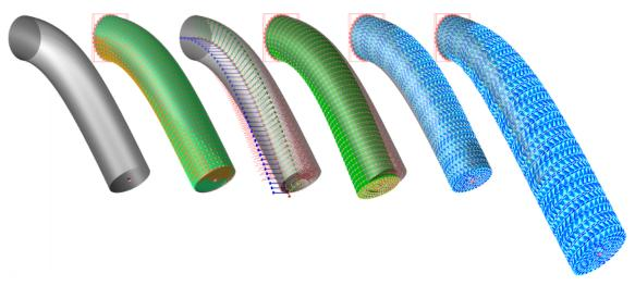
**Figure 1.1** – Simulation results for the different modeling methods. From left to right: the experimental solution, the mass-spring network, the 6-DOF beam, the FEM Hexahedra, the FEM corotational Tetrahedra and the linear FEM Tetrahedra solutions.
