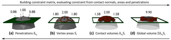
Distributing the constraint pressure as forces over the degrees of freedom
