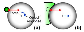
**Figure 4.10** — Responses of a virtual object with the regular god-object method (a) and with our novel God-finger method (b). (a) God-object case, the object rolls. (b) God-finger case, the object slides.
