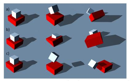
**Figure 1.3** – Fourth test case. A heavy cube (white) is dropped on a light one (dark red), with a scale factor of 1000 on masses. (a) Results with Havok Physics. (b) Results with NVidia PhysX. (c) Results with Bullet Physics. Time step = 1/800s, Friction coefficient = 0.5, Restitution coefficient = 0.4.
