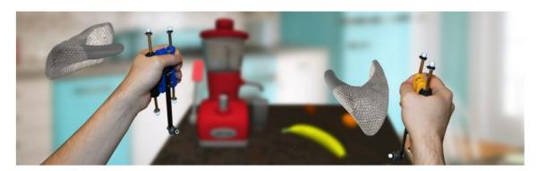
**Figure 9.1** – Illustration of the Virtual Mitten. Each hand holds an elastic device to control a corresponding virtual mitten (in gray) and to grasp virtual objects in a bimanual scenario. The grip force applied by the user is measured to generate pseudo-haptic feedback.
