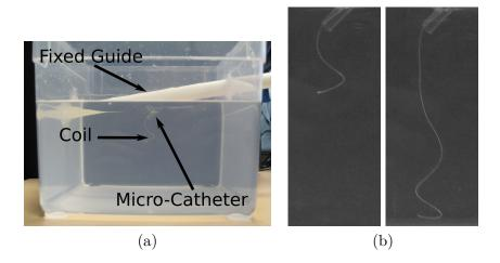
**Figure 3.5** — (a) Experimental setup: the coil is deployed in a contact-free environment. The setup consists of a box filled with water and a transversal fixed guide, defining the path for the catheter. The catheter is first introduced, followed by the helical coil as in the real procedure. (b) Volumetric data is obtained by CT scan and a marching cube is performed to get a mesh of the real coil.
