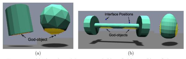
Figure 4.11 - (a) Lifting of virtual objects using only (a) one God-finger or (b) two God-fingers. The contact areas are represented in yellow.
