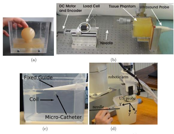
**Figure 1.8** – A selection of phantoms designed during the last years: (a) prostate phantom [Dehghan 07a], (b) needle detection and tracking [Chatelain 13], (c) coil deployment [Dequidt 08] and (d) prostate brachytherapy [Dehghan 07b, Dehghan 08].
