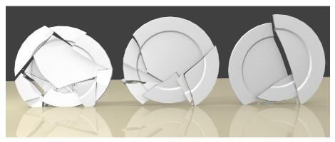
**Figure 2.3** – Effect of damping on the fracture simulation. Our contact force model with modal analysis [Glondu 13] enables to model the inertia and damping of the plate. The left plate has the lowest damping value, letting high frequency modes to propagate and generate many small fragments. The right plate has the highest damping value, generating less fragments.
