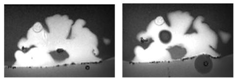
**Figure 1.7** — The brain phantom is imaged with T1-weighted gradient-echo at different inflations.
