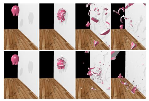
**Figure 2.5** – Snapshots of a simulation of brittle fracture with modal analysis performed without (top) and with (bottom) our database method. Note the recursive fracture of the fragments generated from the first impact on the bottom animation that are not computed in the top animation.
