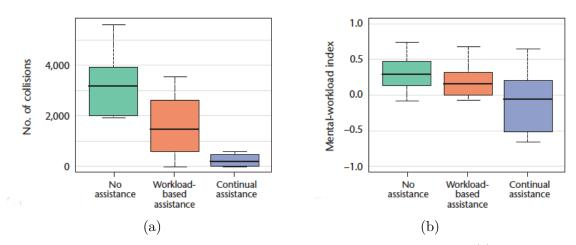
Figure 6.7 – Experimental results obtained with our proof-of-concept setup. (a) Workload-based haptic assistance significantly reduced the number of collisions. (b) It also significantly decreased the mean mental-workload index.
