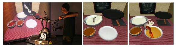
**Figure 4.5** – The virtual crepe preparation simulator: the user pours some batter (a high viscosity fluid) from the bowl and into the pan. The user can feel the forces and torques from the pouring movement, as well as the weight shifting between his hands as the batter goes from the bowl to the pan. Maple syrup could also be poured on the crepe.
