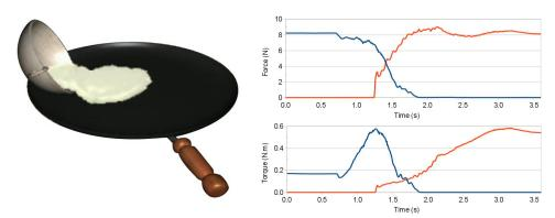
**Figure 4.3** – An illustrative scenario featuring our 6 DoF haptic rendering with fluids. (a) A bowl and a pan, each coupled to a 6 DoF haptic device, are used as containers: fluid is being poured from the bowl into the pan, making the fluid mass shift between both rigid body containers. (b) Plot of the force (top) and the torque (bottom) of the bowl (in blue/dark) and the pan (in red/light) during the pouring motion of some fluid.
