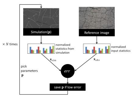
Figure 5.1 — Overview of the optimization process. Parameter vector  $\mathbf{p}$  is optimized iteratively. After each simulation, the statistics of the simulation are compared to the statistics of the reference image. The err function is our metric.
