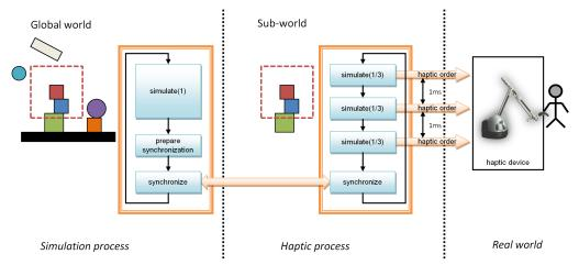
**Figure 4.6** – Haptic-sub world main algorithm. The simulation process simulates the global world once with a time step of dt, while the haptic process simulates for example 3 times its haptic sub-world using a time step of  $1/3 \times dt$ . At the end of the haptic cycle, the two worlds are synchronized, exchanging bodies positions and efforts information.
