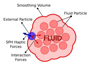
**Figure 4.1** – Smoothing Volume and SPH haptic forces. The Smoothing Volume of a volume of fluid is defined by the sum of the smoothing volumes of each particle belonging to the fluid. When an external particle enters the Smoothing Volume, SPH haptic forces are seamlessly computed between the external particle and the fluid particles whose smoothing volume contains the external particle.
