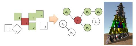
Figure 4.7 – Graph-based haptic sub-world. The graph  $\mathcal{G}$  (middle, containing all nodes) defines the contact configuration of the bodies of the global world. The colored connected components of the graph containing the proxy (in red) form the graph  $\mathcal{H}$  (containing only colored nodes) of the bodies that compose the haptic sub-world. The card house (right) illustrates the haptic sub-world composed of colored cards extracted from the proxy (red card).
