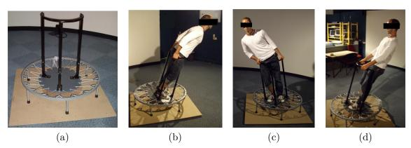
**Figure 8.2** – Illustration of the peripheral device. (a) the device is composed of a basis, a board to support the user and a safeguard. (b, c, d) When using the Joyman, users can stand straight on the board, repealing forces make easy keeping the platform inclination. Users have to lean to start locomotion in virtual worlds. All the leaning directions are possible.
