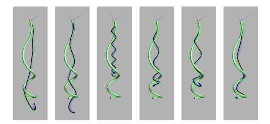
**Figure 3.6** — Illustration of the optimization process to recover rest shape parameters of the coil. The real data are in green while the simulation data are in blue.
