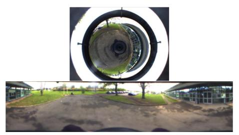
**Figure 8.6** – (Top) Image provided by the catadioptric system. (Bottom) Image displayed in the HMD after its modification.
