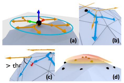
**Figure 4.9** — Steps of the God-finger method. (a) A finger-print is generated as if the object was planar. (b) The contact area is then fit to the geometry of the object. (c) Bumps on the surface are prevented by stopping the scan at sharp edges. (d) The result of the scan is fed back to contact points which describe the contact surface.
