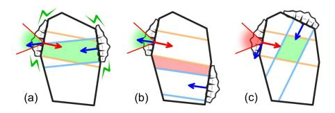
**Figure 9.7** – Different cases of dual contact with a virtual object, case (a) being appropriate for grasping and cases (b-c) not being as such: (a) Normals nearly colinear and hands face-to-face, (b) Hands not in front of each other, (c) Normals far from colinearity.
