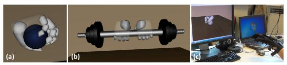
Figure 3.12 – Some object manipulation scenarios with our method. (a) Grasping a rigid ball with all fingers deformable. (b) Lifting a dumbbell with two fully deformable hands. (c) Manipulating a deformable ball using a data glove.
