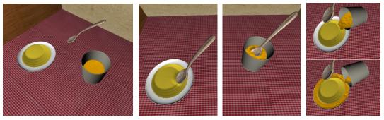
**Figure 4.4** – Scenario illustrating a cooking simulator. The user, through a spoon coupled to the 6DoF haptic device, can touch and play with a custard tart, a glass and its liquid content. Haptic feedback is seamlessly computed for the three states of matter simultaneously.
