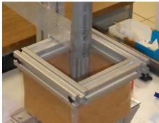
Figure 2.7 – One of the test benchmark we designed for our validation experiments. Left: overview of the bench, a ball is dropped in the tube to fall on a tile set up on its support. Right: zoom on the aluminum support of the tile. To design a 4 punctual contacts test, 4 metallic balls were fixed on the top of the aluminum support.
