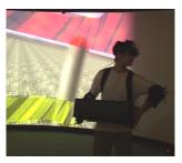
Figure 10.1 – The Magic Barrier Tape displays the boundaries of the real workspace as a virtual barrier tape, and uses a hybrid position/rate control to travel in the VE. The user (left) "pushes" on the Magic Barrier Tape (center) to move inside the VE when he reaches the workspace boundaries. Any tracked body part can be used to trigger the Magic Barrier Tape (right).
