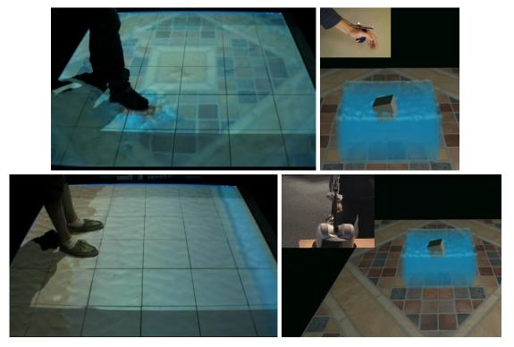
**Figure 6.2** – Interaction examples using different body parts and rendering devices: a foot-water pool scenario using actuated tiles (left, top), a user feeling the water under his feet as a wave washes up on the beach using actuated tiles (left, bottom), and a hand-water basin scenario using a small vibrator (right, top) or a 6DoF haptic device (right, bottom).
