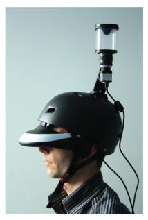
Figure 8.5 – Ilustration of the FlyVIZ prototype.
