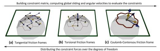
**Figure 3.9** – Formulation of Coulomb-Contensou friction for the contact surface with our approach. (a) Individual Coulomb friction frames with sliding velocities at each contact point. (b) Torsional velocities evaluated from vectors orthogonal to the contact surface
