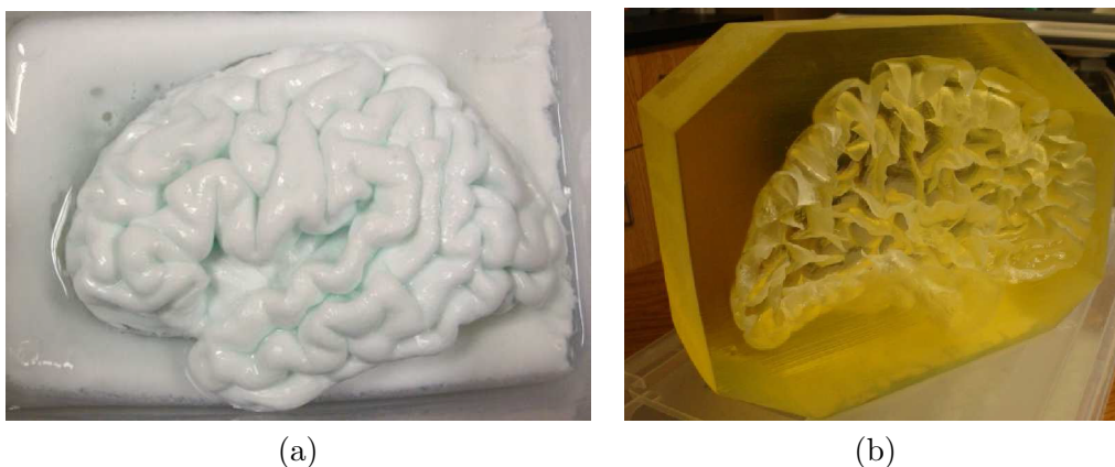
Figure 1.5 – (a) The PVA-C phantom casted from the Colin27 based brain phantom mold using our PVA solution. The deep sulci as well as the insular regions are represented in the phantom. (b) The flexible mold used for obtaining the phantom.
